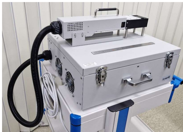
Figure 7. Photograph of the fabricated D-band THz A-scanner, with a 30 cm ruler included for scale reference.
