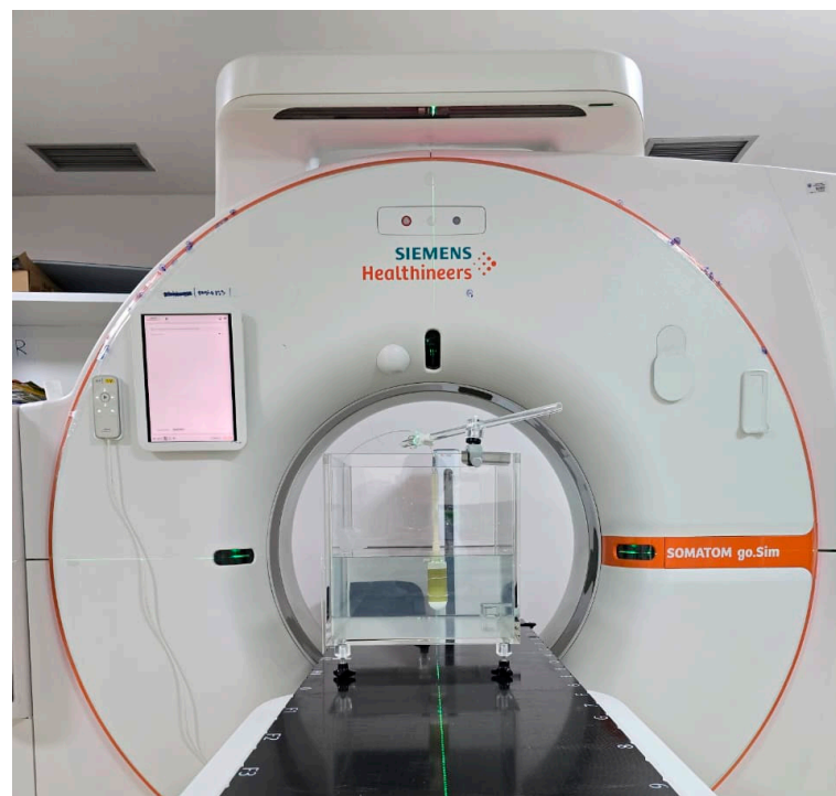
Figure 2. Computer Tomography (CT) simulation of applicator with EBT3 film inside of water phantom.
