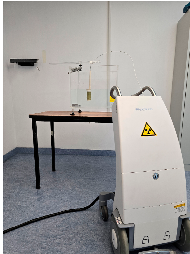
Figure 4. The HDD Flexitron afterloader and applicator with wrapped EBT3 in water phantom during irradiation.
