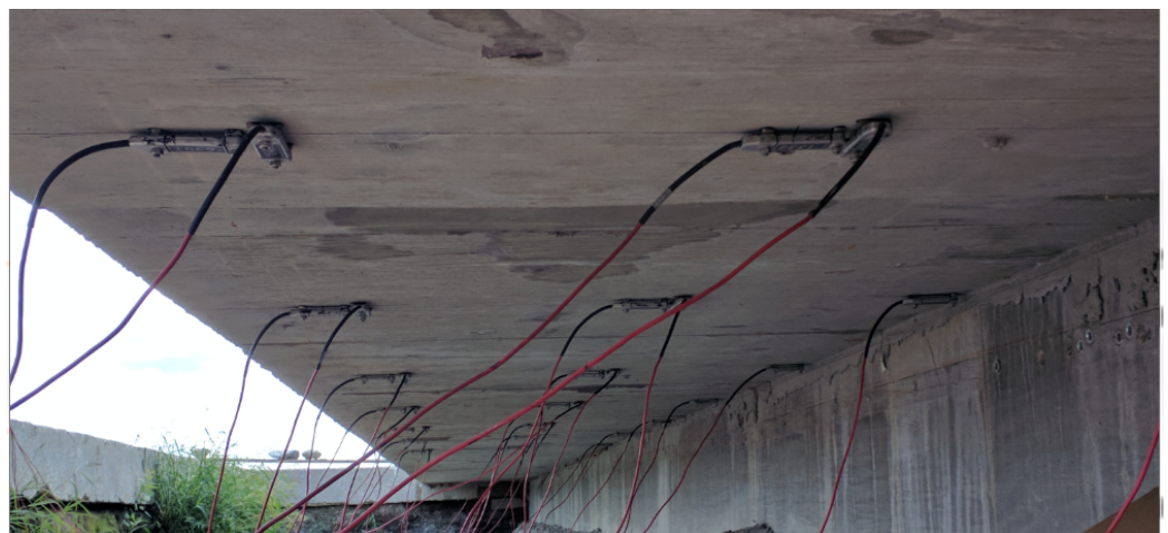
Figure 2. Sensors installed on the underside of the bridge deck for structural health monitoring.
