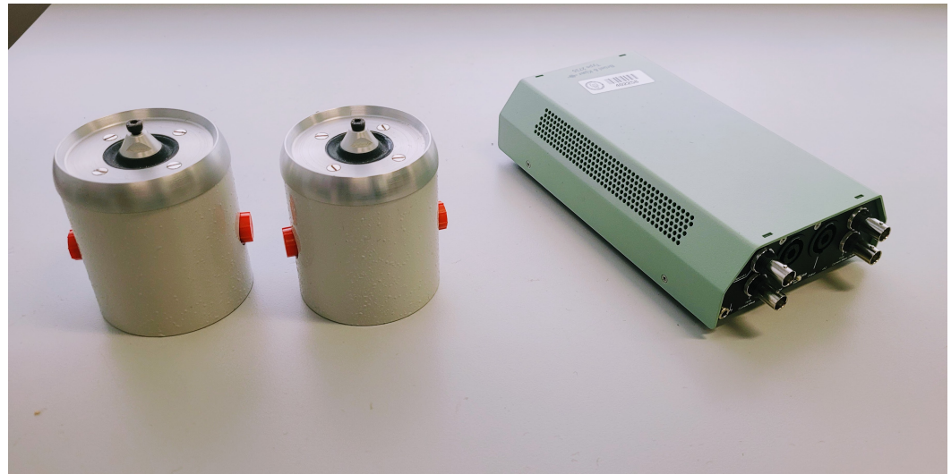
Figure 2. LDS 201/3 shakers and signal amplifier model 2735.
