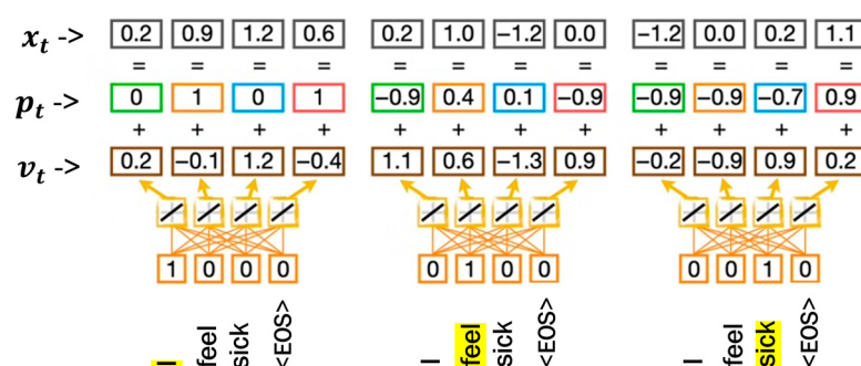
Figure 4. Vector containing embedding and positional information.
