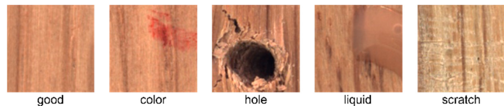
Figure 3. Types of good and defective wood patterns.
