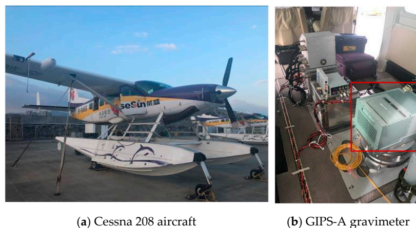
Figure 3. Installation of the GIPS-A gravimeter in an amphibious Cessna 208 aircraft.
