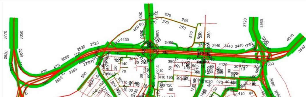
Figure 1. Maximum traffic peak (veh./h) on bridges for 2020 with CPTS [13].
