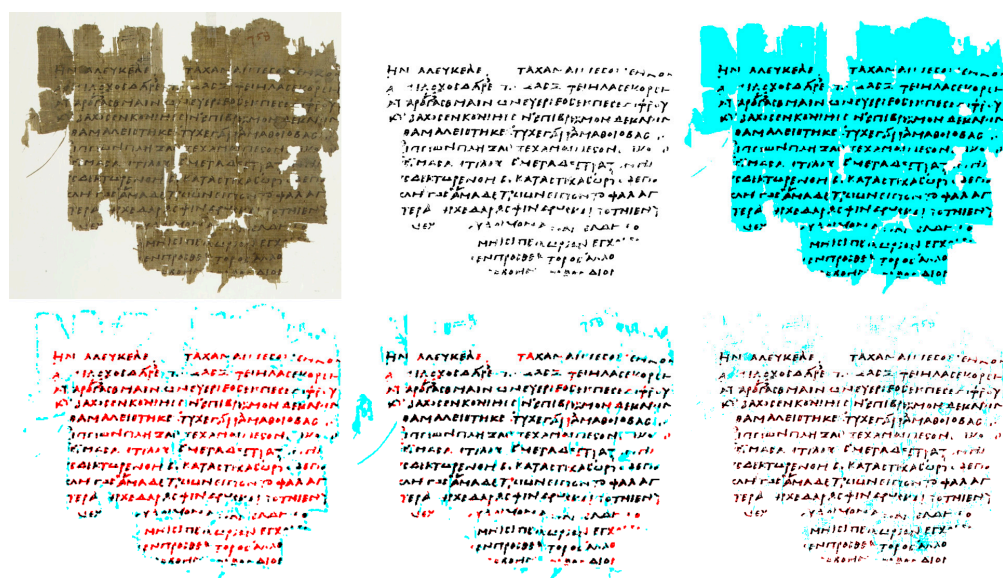
Figure 2. From top to bottom, left to right: original image, ground truth, Otsu binarization, Sauvola binarization, GDB binarization, proposed solution binarization.
