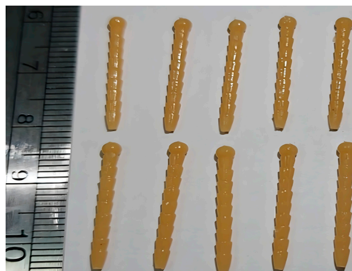
Figure 14. Injection-molded PLA/PCL/ACP dental posts for deciduous teeth, produced using the optimal processing parameters (A1B2C3). A ruler is included for scale.
