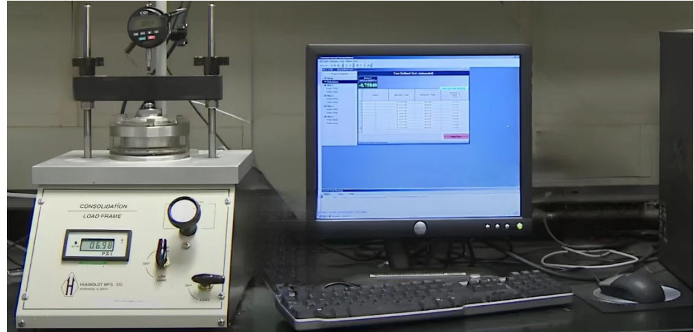
Figure 3. Consolidation test apparatus showing the loading frame, consolidation cell, and dial gauge.
