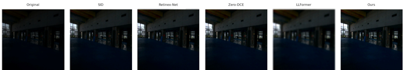
Figure 6. Visual comparison on an unseen low-light image from a DICM-style dataset. Our model (rightmost) achieves enhanced brightness, natural color balance, and better contrast relative to prior methods, confirming its generalization to real-world low-light conditions beyond the training distribution.
