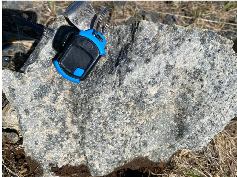
Figure 3. A norite specimen displaying its coarse texture.
