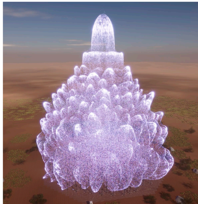
Figure 5. 3D representation of the power pattern from the simulated array shown Figure 3. Credits: ICRAR/INAF.
