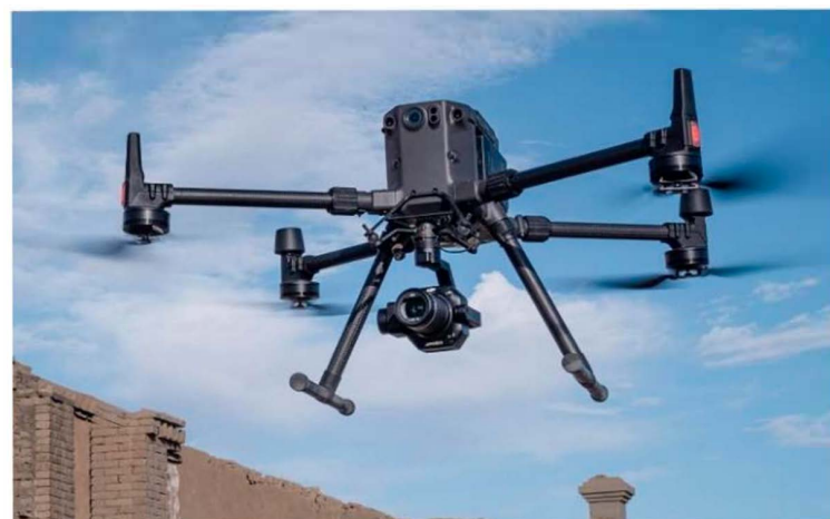
Figure 1. DJI Matrix 300 RTK unmanned aerial vehicle.
