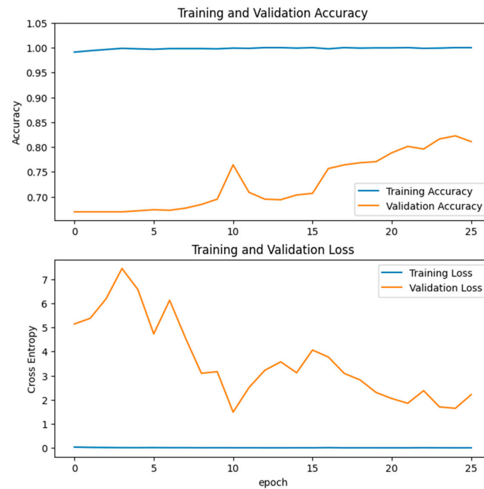
Figure 5. Training and validation loss and accuracy for the case of the base model with the 10 last layers being unfrozen.
