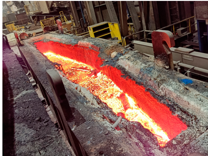
Figure 28. No visible wearing of the working lining after 18 heat cycles in the slag line area using experimental configuration SP-K4 (impact pad SPHERIC K4).
