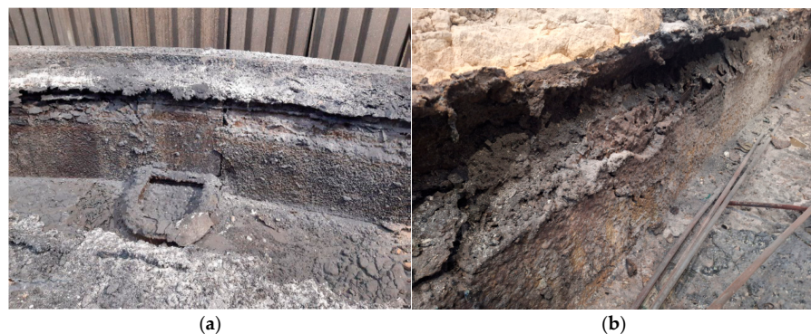
Figure 27. Wearing of the working lining after 18 heats in the slag line area: reference configuration K (a) and detail image (b).
