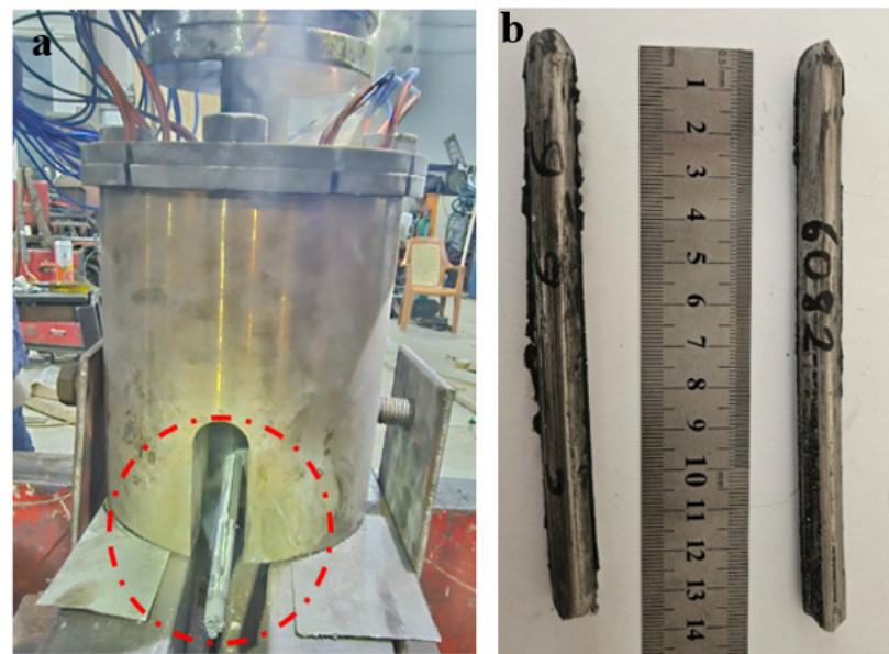
Figure 16. (a) View of the workpiece (red dashed line) emerging through the exit channel during the Vo-CAP process. (b) Vo-CAP-processed AA6082.
