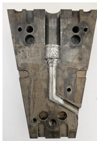
Figure 17. Deformation path geometry in Vo-CAP die.
