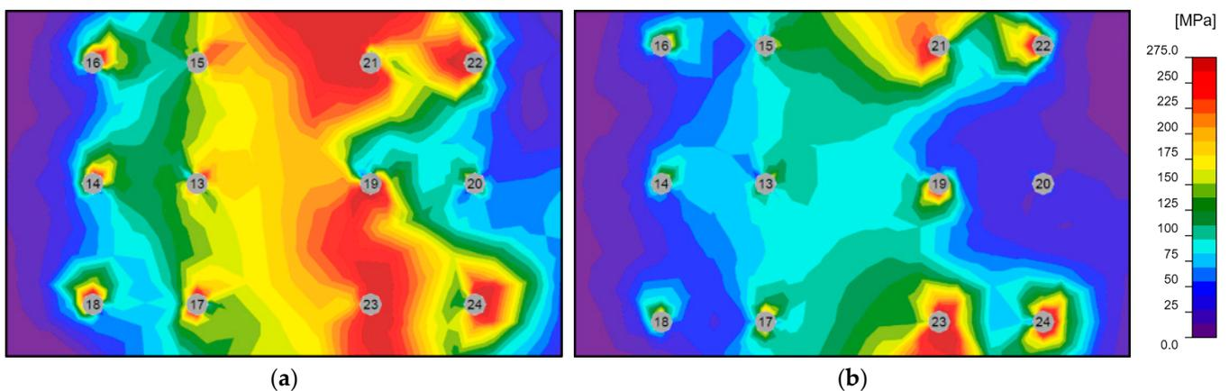
**Figure 6.** von Mises stress distribution in plates with color scale: (a) 3 mm thick plate and vertical spacing of 70 mm; (b) 5 mm thick plate and vertical spacing of 80 mm. The numbering of bolts is indicated.
