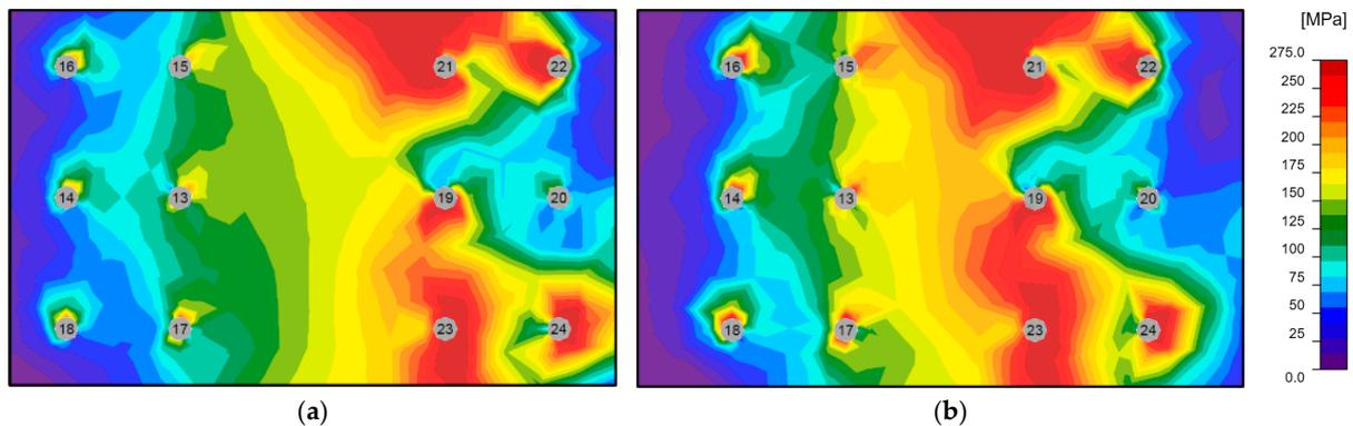
Figure 11. von Mises stress distribution in plates with color scale: (a) 3 mm thick plate with 30 mm horizontal spacing to the vertical edge; (b) 3 mm thick plate with 50 mm horizontal spacing to the vertical edge. The numbering of bolts is indicated.
