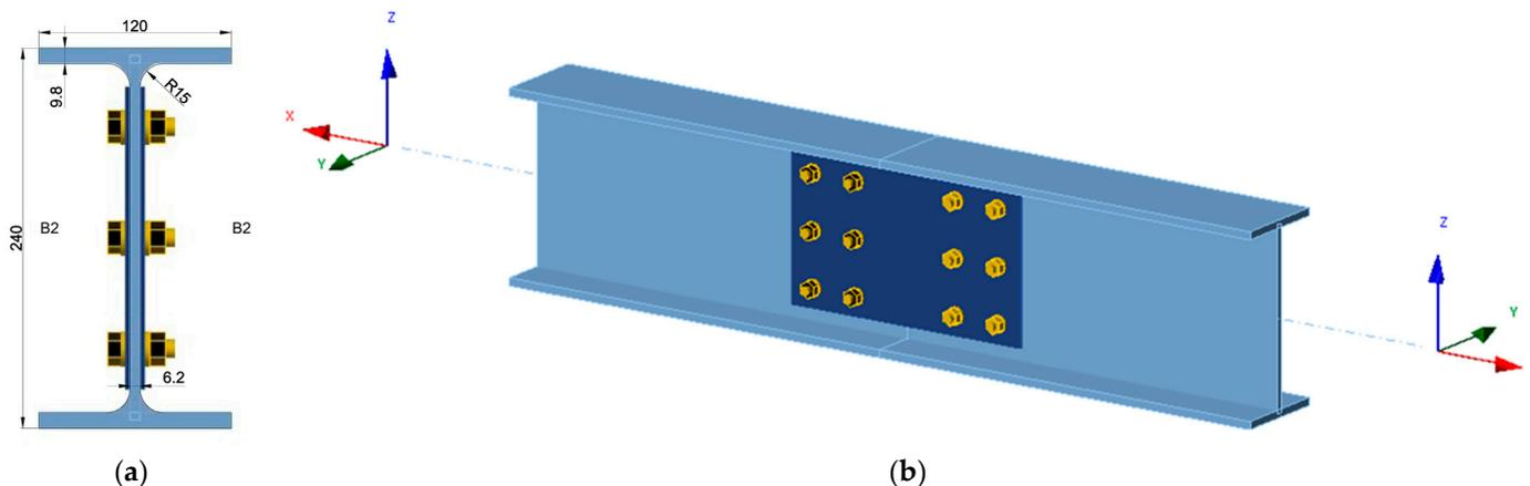
**Figure 1.** Joint components: (a) Cross-section view with dimensions in mm; (b) axonometric view.
