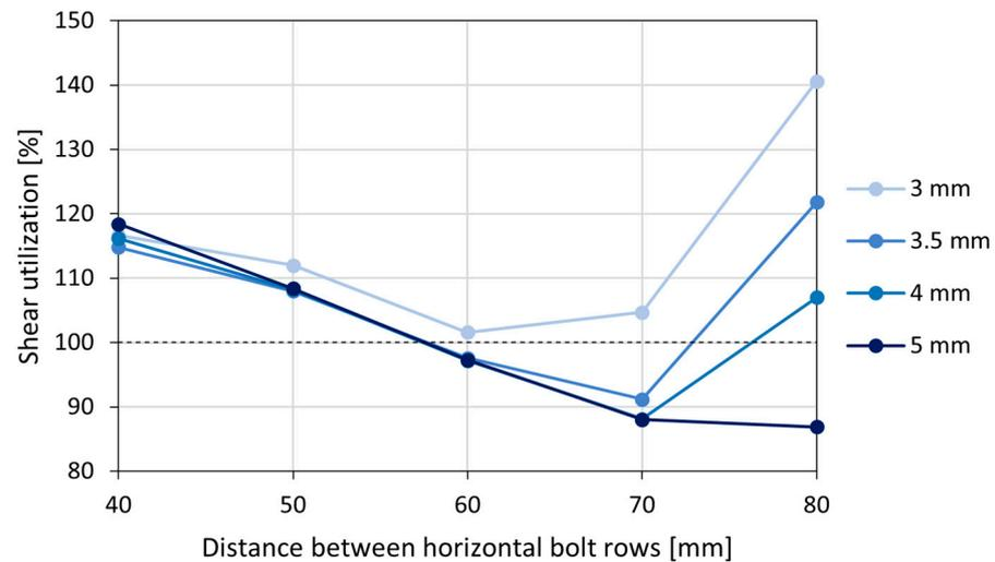
Figure 14. Bolt shear utilization for horizontal spacings of 50–60 mm with offset in central row.
