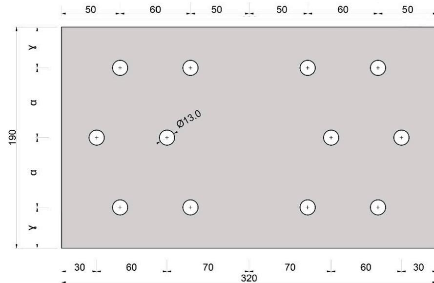
Figure 12. Dimensions of steel plate and position of holes with offset in central row.
