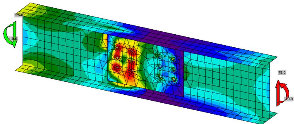
**Figure 2.** Joint model in IDEA StatiCa using finite elements with the range of colors representing the state of internal tensions.
