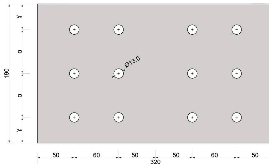
**Figure 3.** Dimensions of steel plate and position of holes.
