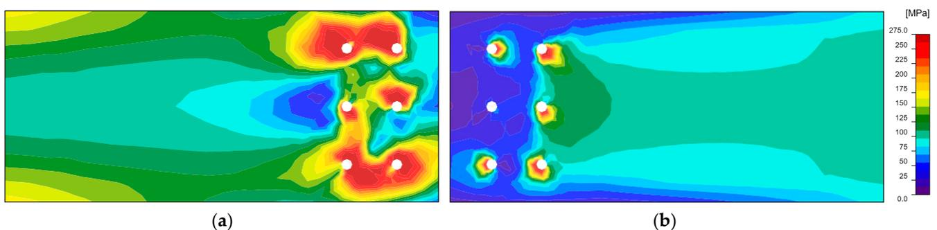
**Figure 7.** von Mises stress distribution in the web of IPE240 profiles with color scale: (a) left end; (b) right end.
