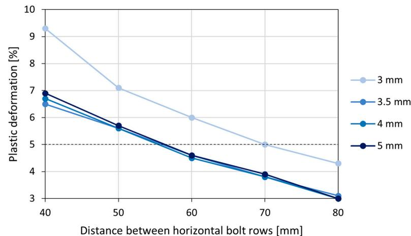
Figure 13. Equivalent plastic maximum deformation for horizontal spacings of 50–60 mm with offset in central row.
