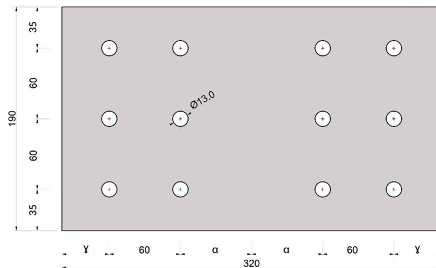
**Figure 9.** Dimensions of steel plate and position of holes with varying horizontal spacing.
