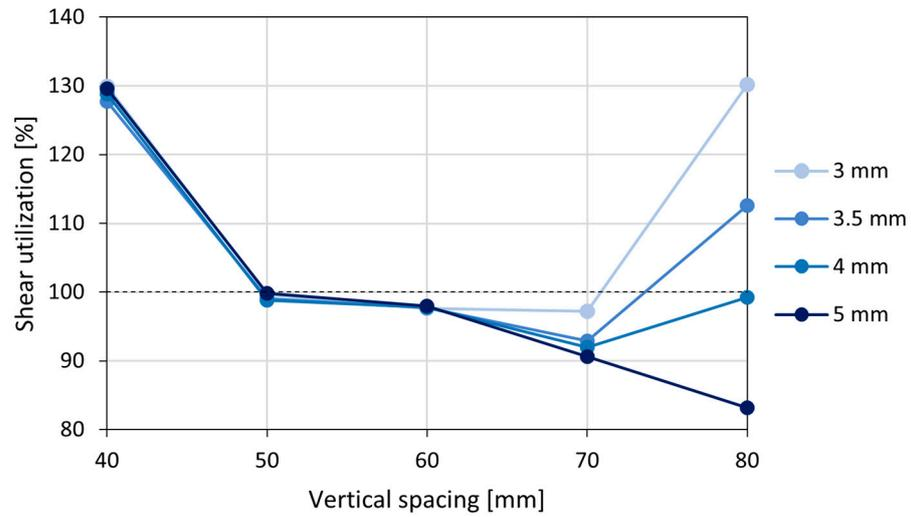
**Figure 8.** Bolt shear utilization for horizontal spacing of 50–60 mm.
