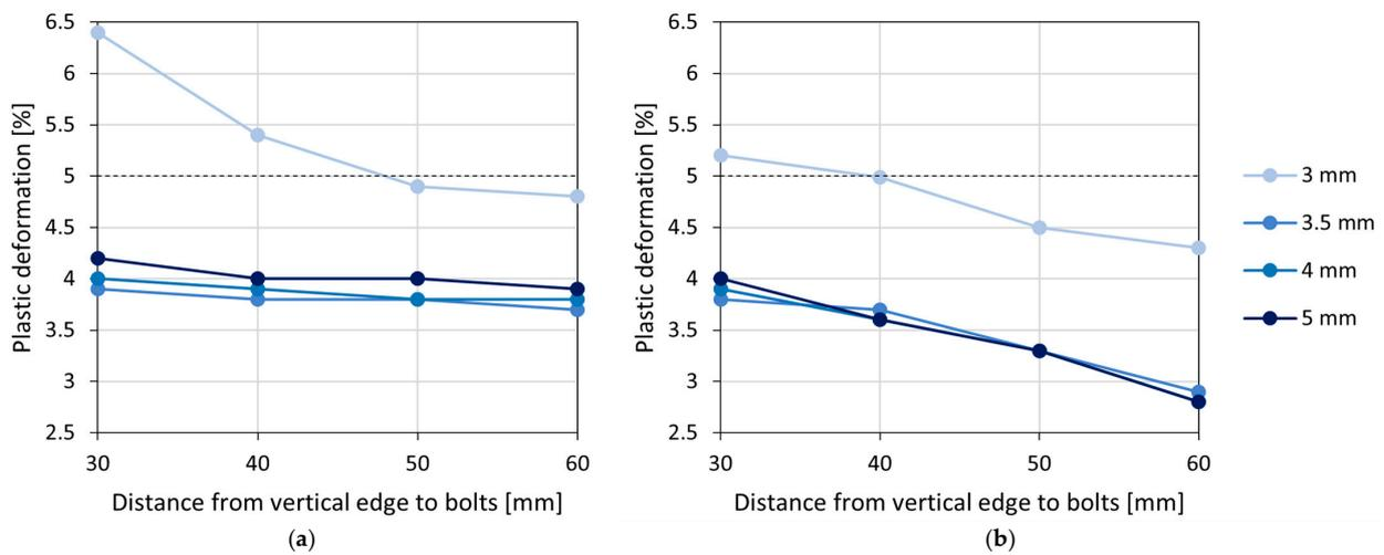
Figure 10. Plastic deformation: (a) 60 mm vertical spacing; (b) 70 mm vertical spacing.
