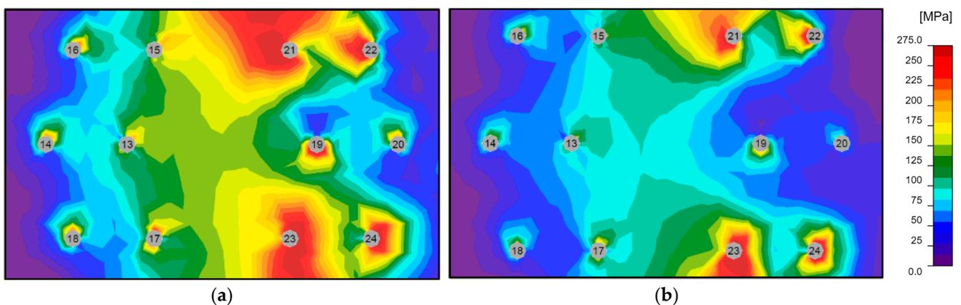
Figure 15. von Mises stress distribution in plates: (a) 3.5 mm thick plate with 60 mm vertical spacing between row bolts; (b) 5 mm thick plate with 80 mm vertical spacing between row bolts. The numbering of bolts is indicated.
