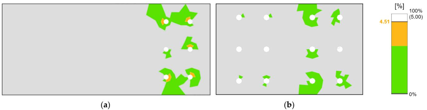
**Figure 5.** Verification of plastic deformation in joint with 3 mm thick plate with vertical spacing of 70 mm: (a) IPE240 web; (b) plate.
