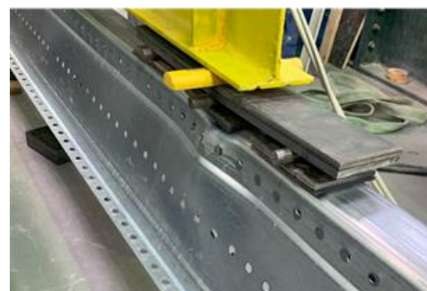
Figure 8. Failure modes observed during the testing of the 300 \times 2.5 profile.
