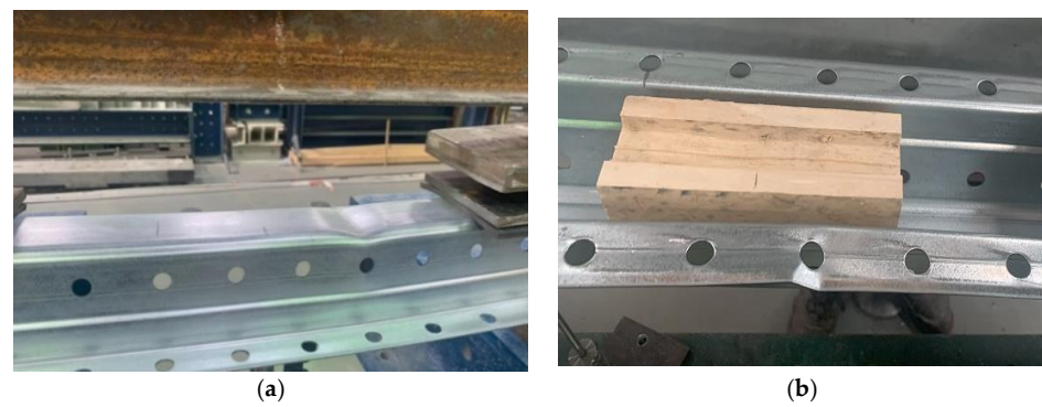
Figure 6. Failure modes observed during the testing of the 70 \times 1.5 profile under (a) a downward load and (b) an upward load.
