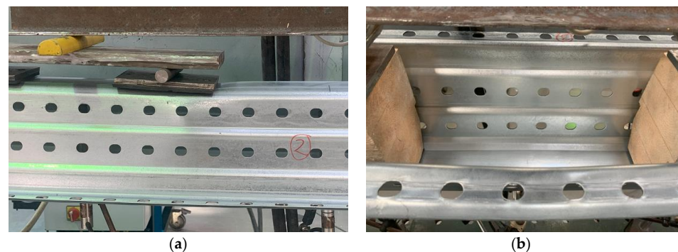
Figure 7. Failure modes observed during the testing of the 170 \times 2.0 profile under (a) a downward load and (b) an upward load.
