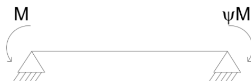
Figure 20. Scheme of the loading pattern.
