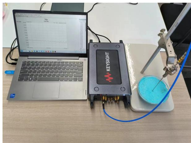
Figure 9. Dielectric constant measurement.
