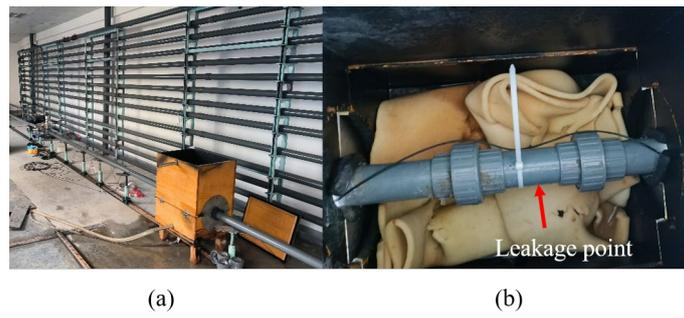
Figure 5. (a) Simulating water pipeline; (b) leakage point.
