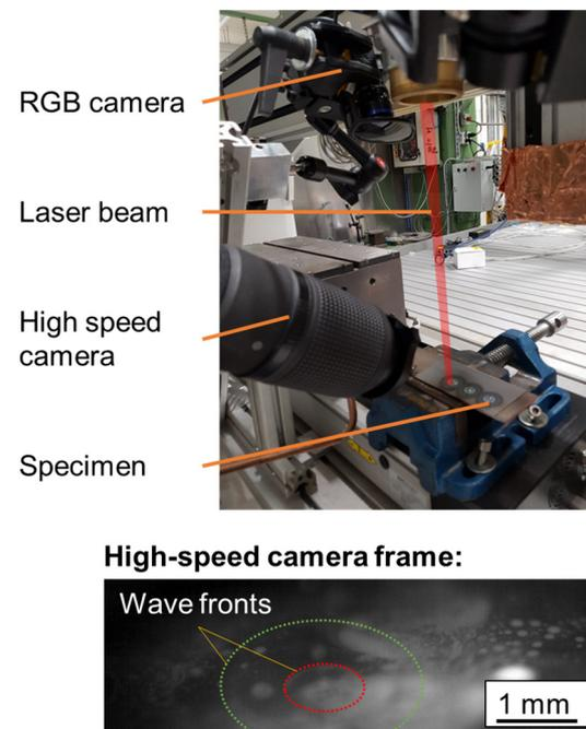
**Figure 1.** Set-up to create a controlled melt pool using laser beam heating, observed by an RGB camera for temperature calculations and a high-speed camera to observe melt pool surface wave propagations.
