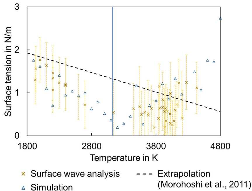
Figure 5. Surface tension measurements and calculations around the boiling temperature of steel, including surface wave analysis, simulation results and extrapolation from Equation (1) [24].
