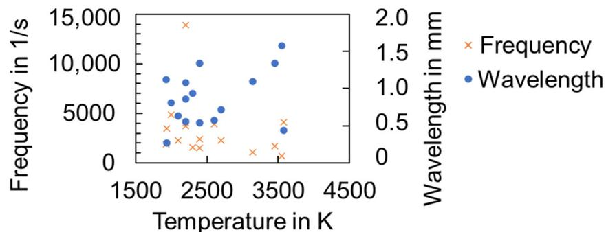
Figure 3. Measurements of surface wave frequencies and wavelengths at multiple temperatures.
