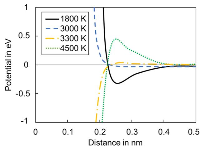
**Figure 6.** Pair potentials used in the ion calculation below and above boiling temperature.
