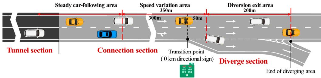
**Figure 4.** Zonal classification of diverging area based on the vehicle speed attributes. The sign displayed feature Chinese characters for specific geographical locations (Jingyang, Xianyang, yan, etc.) pertinent to the study’s context in China and presented in their native script for accuracy.
