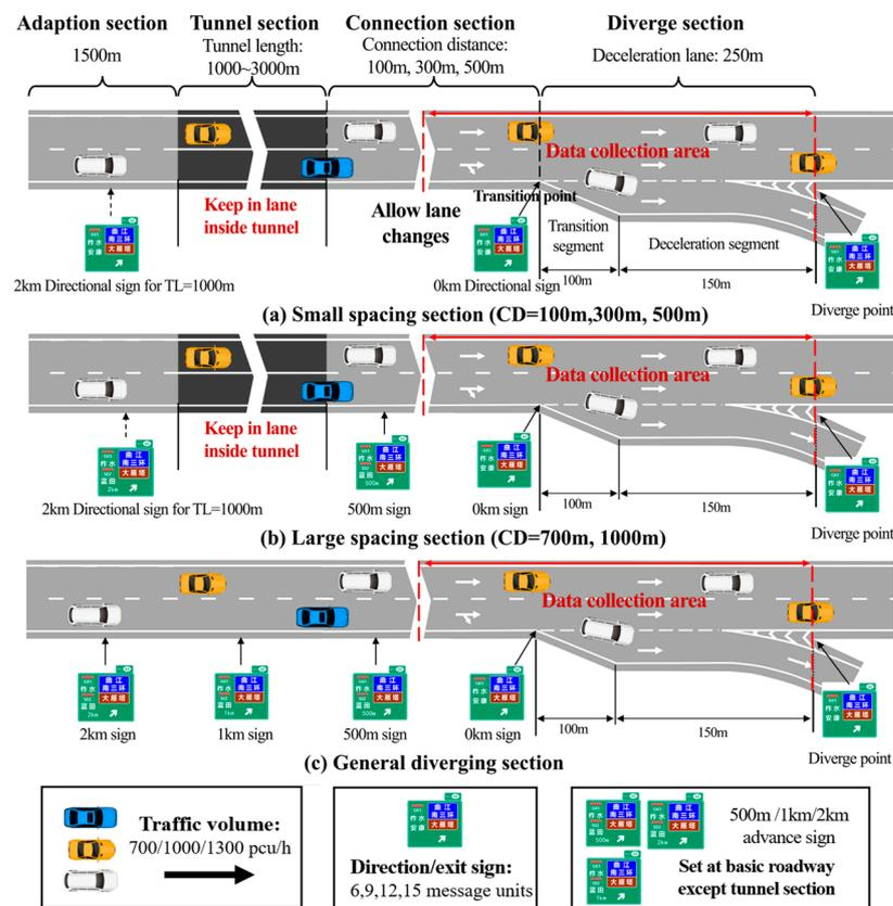
**Figure 2.** Roadway design and sign setting under the simulated scenario. The signs displayed feature Chinese characters for specific geographical locations (Zhashui, Ankang, Qujiang, etc.) pertinent to the study’s context in China and presented in their native script for accuracy.
