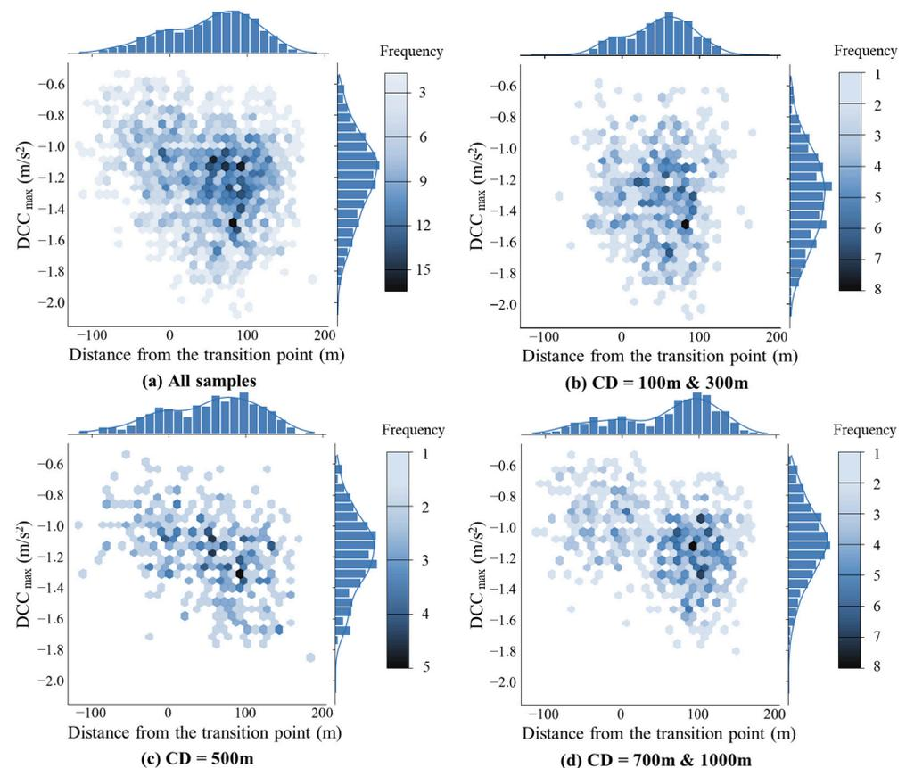
Figure 8. The distribution of maximum deceleration position.
