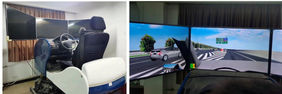
**Figure 1.** Six-degrees-of-freedom vehicle motion simulation platform.
