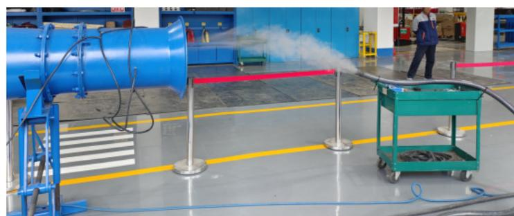
**Figure 7.** Dust removal performance test.
