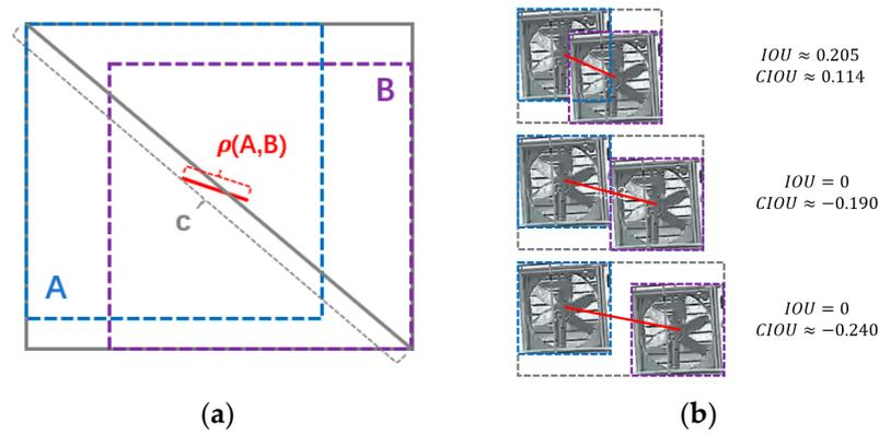
**Figure 7.** (a) CIOU schematic diagram; (b) comparison of IoU and CIOU in different overlapping situations.
