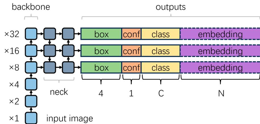
**Figure 1.** The reduction of feature maps across YOLOv7. The dashed boxes in the figures signify changes introduced in our study, elaborated in subsequent sections.
