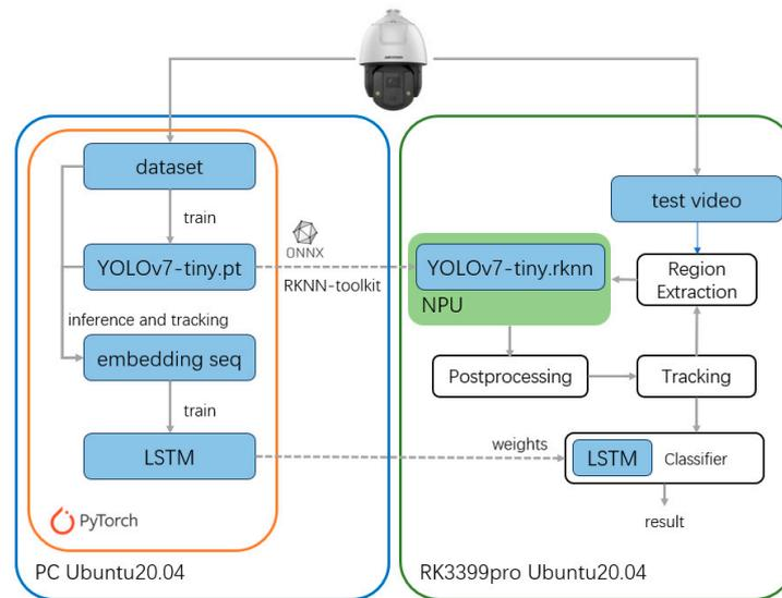
Figure 8. Experimental setup.
