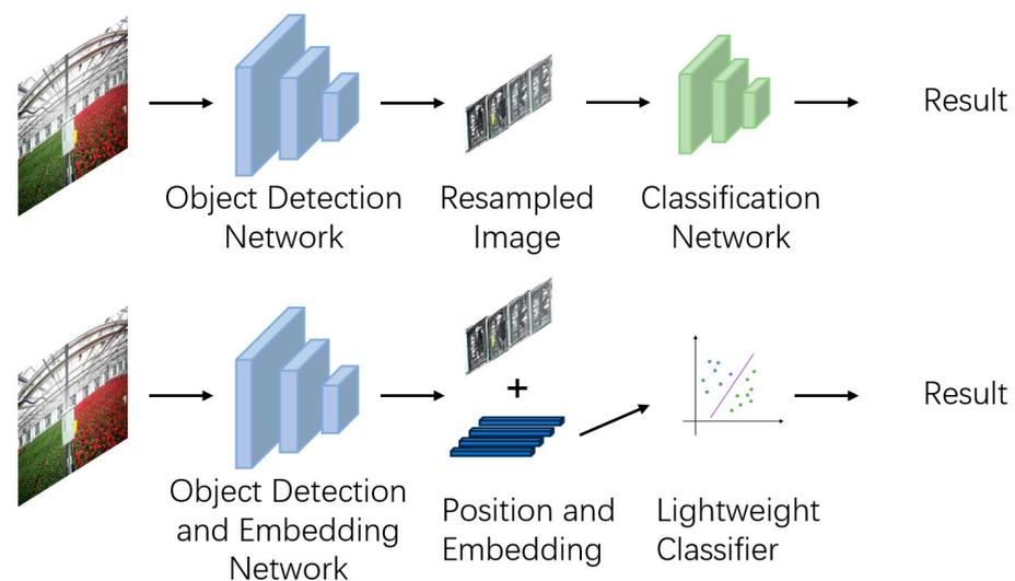
**Figure 3.** A comparative analysis of inference methodologies: traditional vs. integrated detection-embedding frameworks.
