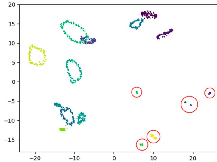
**Figure 11.** The distribution of embedding after PCA. Each colored dot represents an embedding. The dots in the red circles represent the stopped fans.
