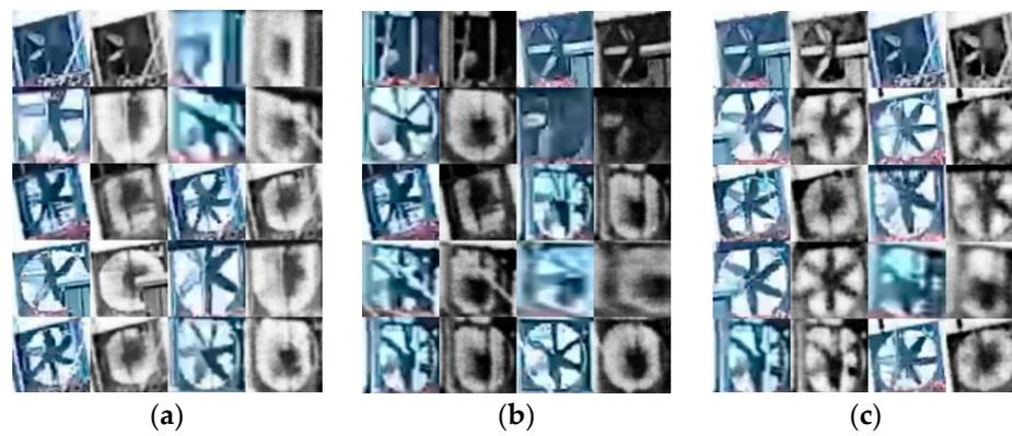
**Figure 10.** Impact of enhancement techniques on image reconstruction. The colored image is the original image, and the grayscale image is the reconstructed image. (a) Normalization; (b) gamma transformation; (c) histogram equalization.
