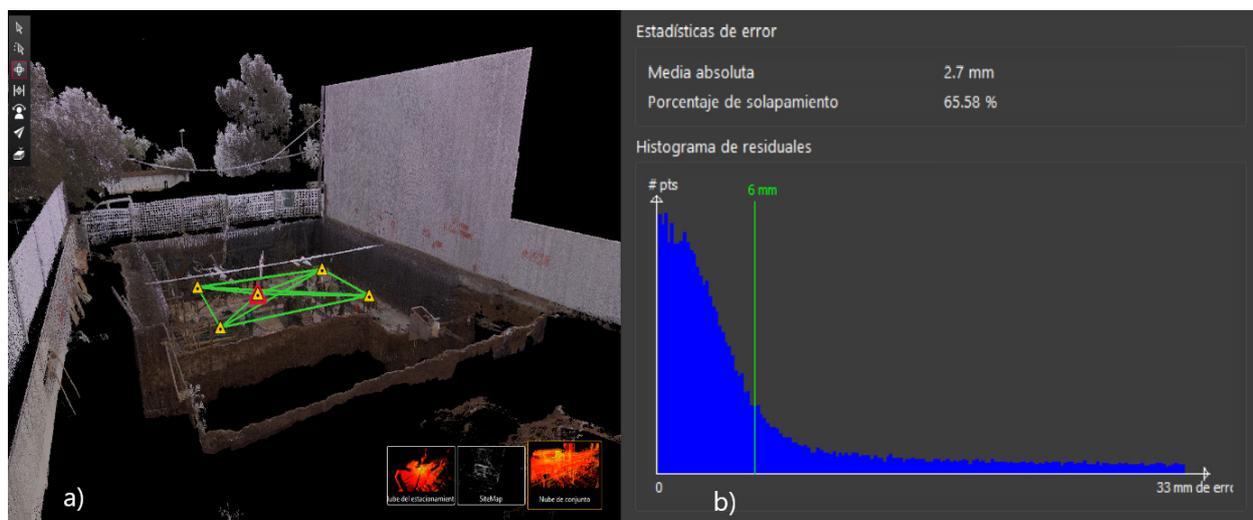
Figure 3. (a) Point Cloud parking link and (b) Link result of Cyclone 3DR 360 scans.
