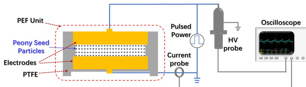
**Figure 1.** Schematic diagram of PEF processing experiment.
