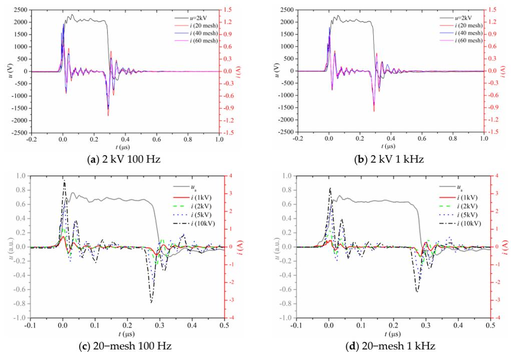
Figure 4. Voltage and current waveforms during the process of PEF treatment on peony seeds.
