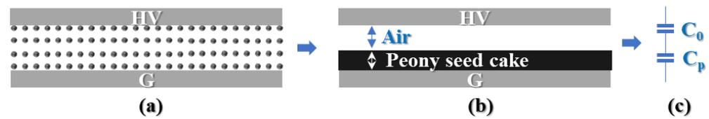
**Figure 5.** Equivalent circuit of PEF treatment unit for peony seeds: (a) peony seeds of different particle sizes are filled in the processing unit; (b) assuming that the peony seed particles are compacted into cakes; (c) equivalent model of capacitors connected in series.
