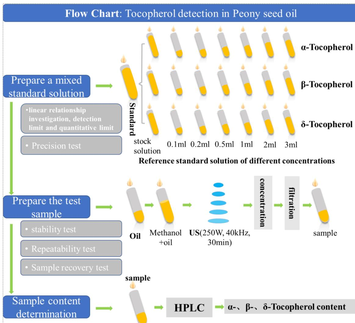
Figure 3. Flow chart of tocopherol detection.
