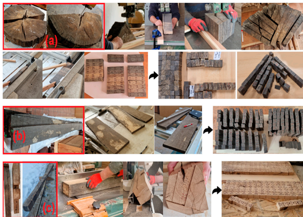
Figure 1. Types of wood material and phases of test samples preparation: (a) log cross sections (SO_S2a, SO_S2b), (b) timber pieces (SO_S1, SO_S3) and (c) elements of aged wood recovered from constructions (AO_C).
