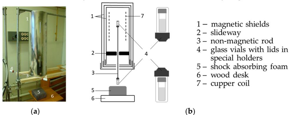
**Figure 1.** Vertical unit for vigorous shaking of water under various magnetic conditions (GMF, near-zero magnetic field, or CMF): (a) general view; (b) schematic drawing [11].
