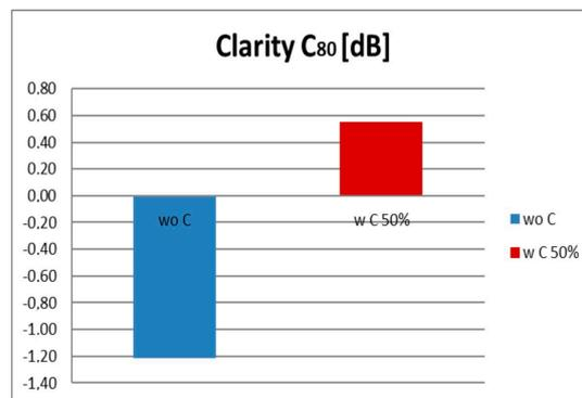
**Figure 9.** Average clarity index,  $C_{80}$ , without curtains (wo C) and with 50% curtains (w C 50%) down on the lateral walls.
