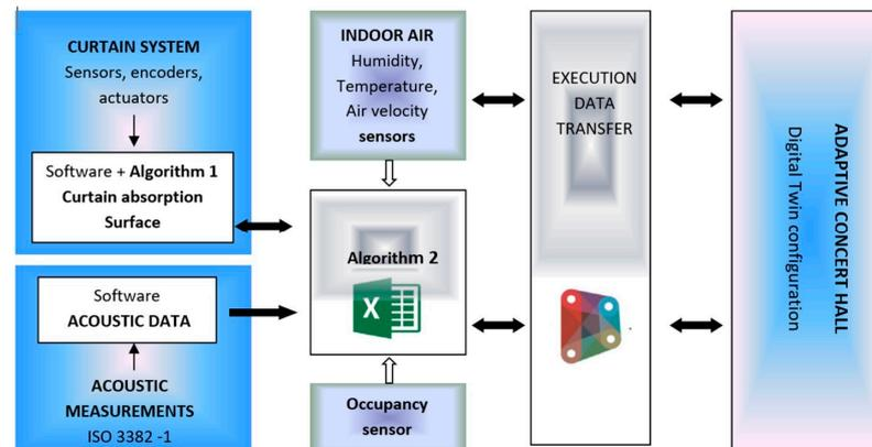
**Figure 3.** Integrated digital twin framework (VPL Dynamo version 2018, Excel version 2016).
