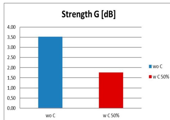
**Figure 10.** Average strength index,  $G$ , without curtains (wo C) and with 50% curtains (w C 50%) down on the lateral walls.
