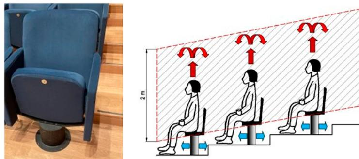
**Figure 11.** Single seat diffuser and heat load definition by volumetric heat source.
