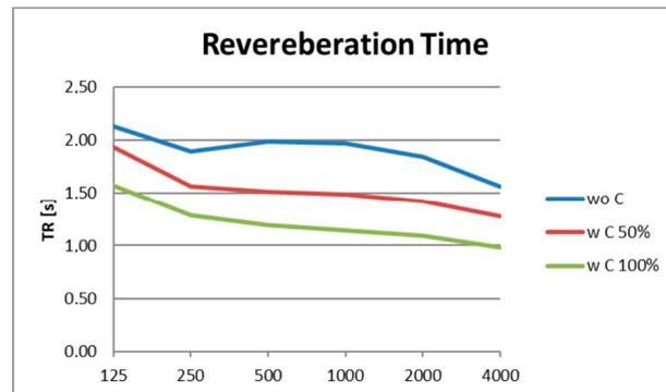
**Figure 8.** Average reverberation time without curtains (wo C), with 50% curtains (w C 50%), and with 100% curtains (w C 100%) down on the lateral walls, homogeneously distributed.
