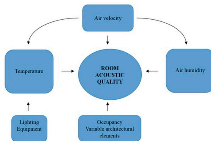
**Figure 1.** Main factors that directly and indirectly influence the room acoustic response.
