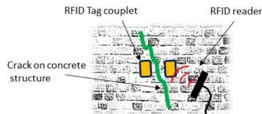
**Figure 17.** Envisaged system layout: an RFID reader wirelessly interrogates [34].
