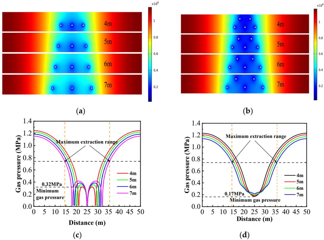
**Figure 14.** Gas pressure distribution and change curve of different drill hole spacing and multi-row drill hole arrangements. (a) Gas pressure distribution in single row of holes. (b) Gas pressure distribution in double row of holes. (c) Variation curve of gas pressure in a single row of holes. (d) Variation curve of gas pressure in double row of holes.
