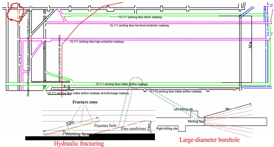
**Figure 15.** Design layout of drill holes on-site at the working face.
