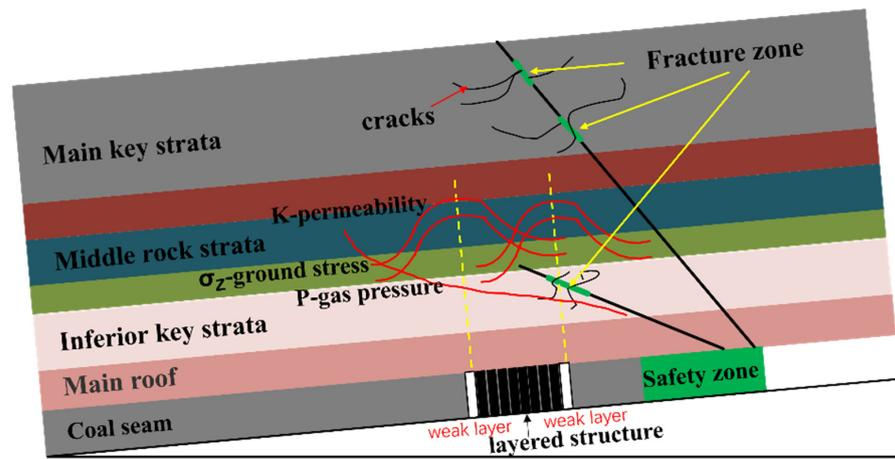
Figure 1. Structural model of laminated combined coal rock body.
