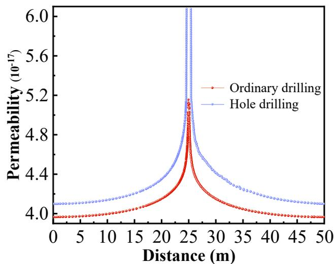
**Figure 8.** Variation in permeability around boreholes.
