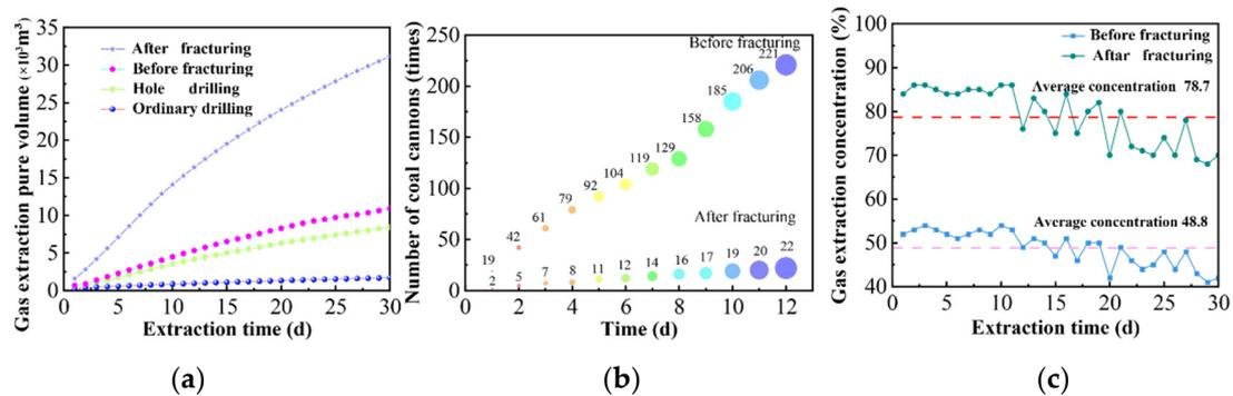
**Figure 16.** Changes in pure volume of gas extraction and extraction concentration before and after fracturing of key strata. (a) Gas extraction. (b) Cumulative number of coal cannons before and after fracturing. (c) Gas extraction concentration before and after fracturing.
