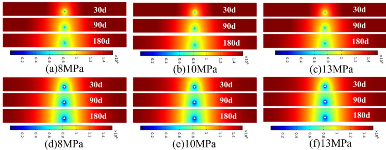
Figure 10. Gas pressure distribution under different overburden stresses.
