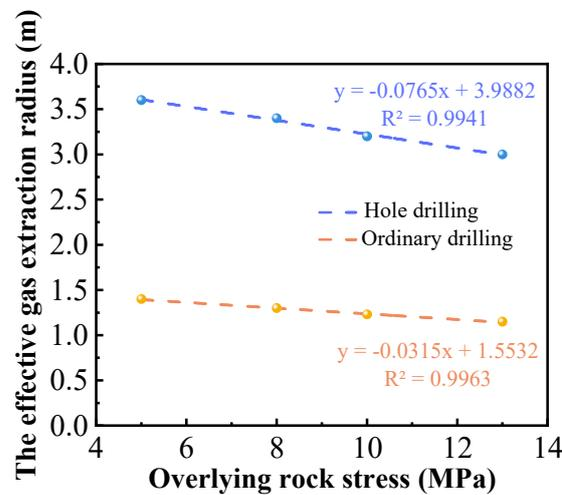
Figure 13. Fitting curve between effective gas extraction radius and overburden stress.
