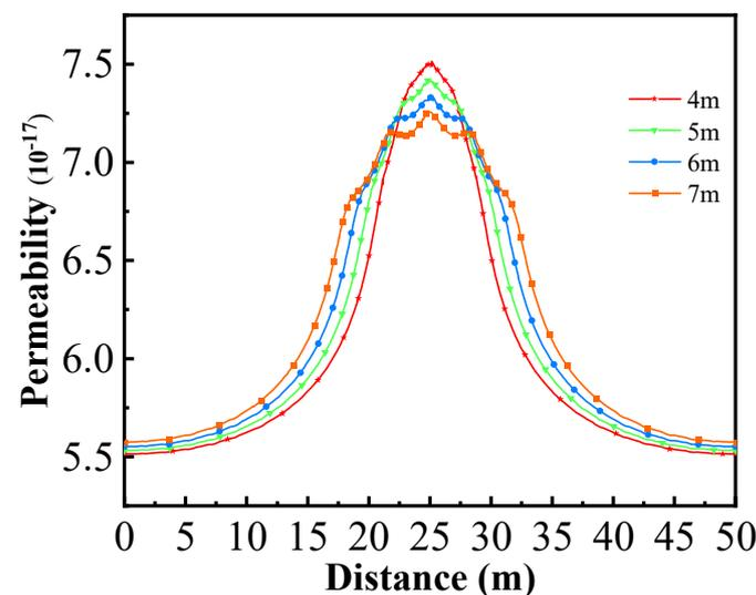
Figure 9. Variation in coal seam permeability.
