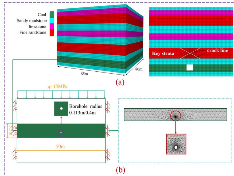
**Figure 4.** Model building and meshing. (a) Overburden fracturing model. (b) Geometric model of gas extraction.
