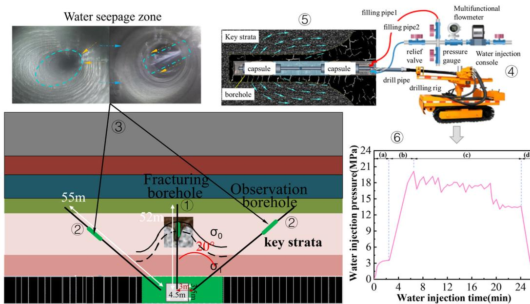
Figure 3. Design and test of fracturing scheme for overlying strata.
