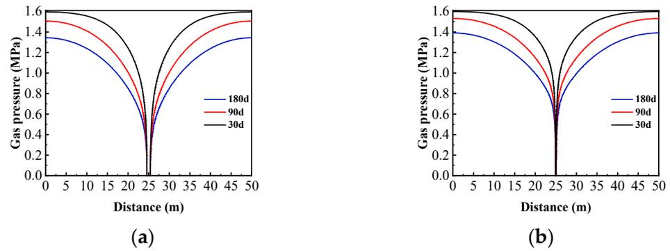
Figure 12. Variation curve of extraction time and gas pressure. (a) Hole drilling. (b) Ordinary drilling.
