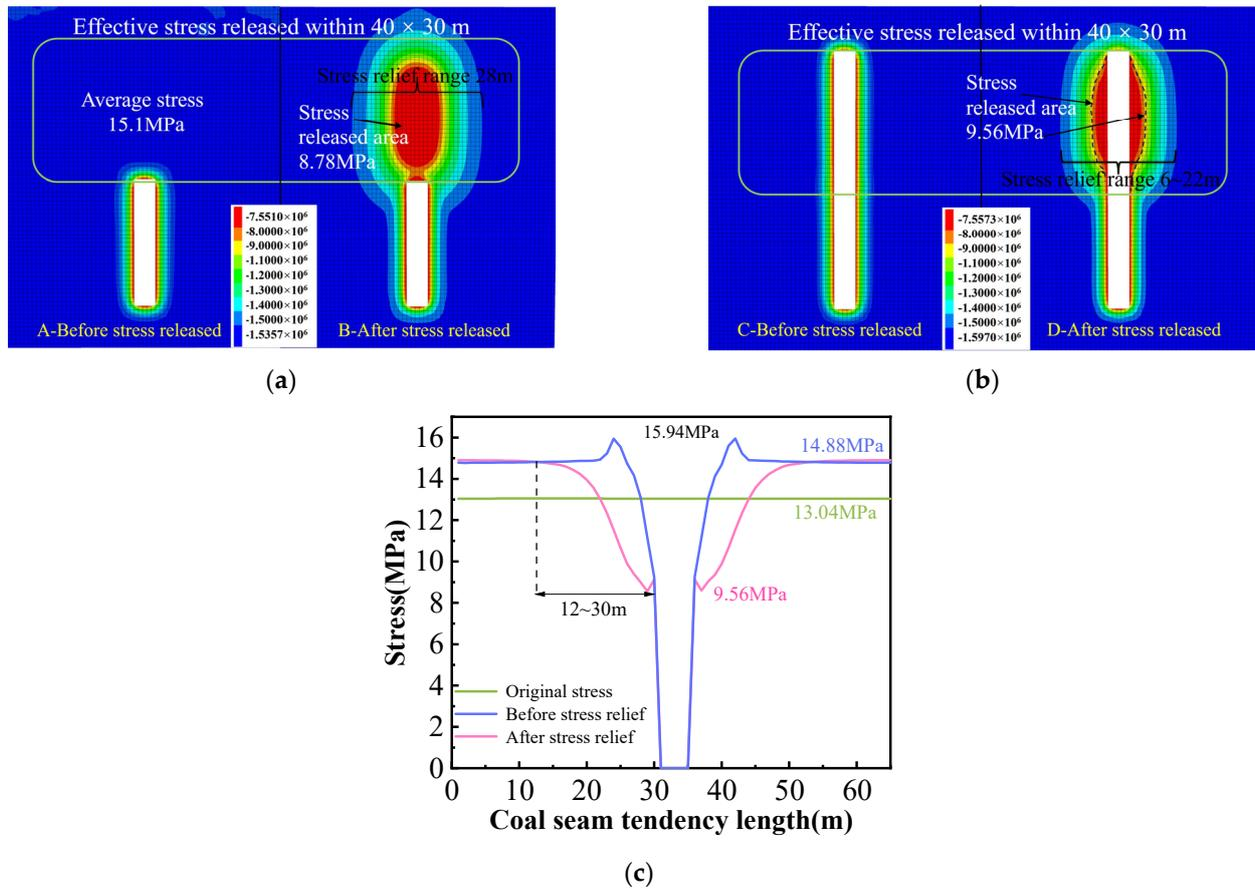
**Figure 5.** Stress change rule of coal seam before and after unloading of key strata. (a) Advanced stress nephogram of coal seam. (b) Stress nephogram after coal seam excavation. (c) Stress curve after coal seam excavation.
