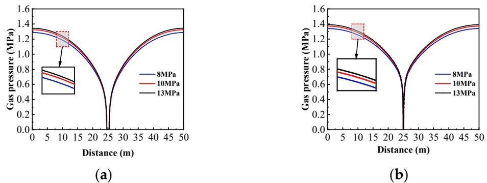
Figure 11. Variation curve of overlying rock stress and gas pressure overlying rock layers. (a) Hole drilling. (b) Ordinary drilling.
