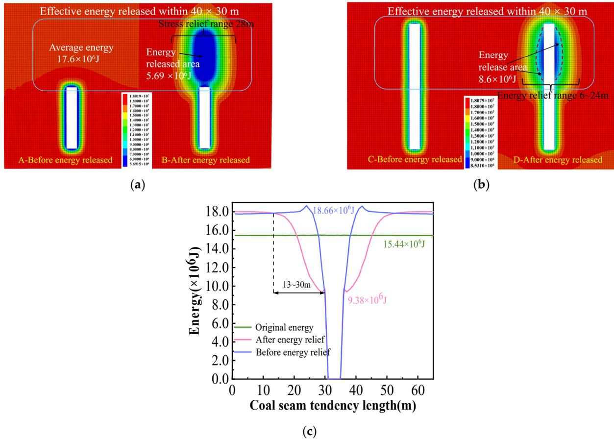
**Figure 6.** Energy change rule of coal seam before and after unloading of key strata. (a) Advanced energy nephogram of coal seam. (b) Energy nephogram after coal seam excavation. (c) Energy curve after coal seam excavation.
