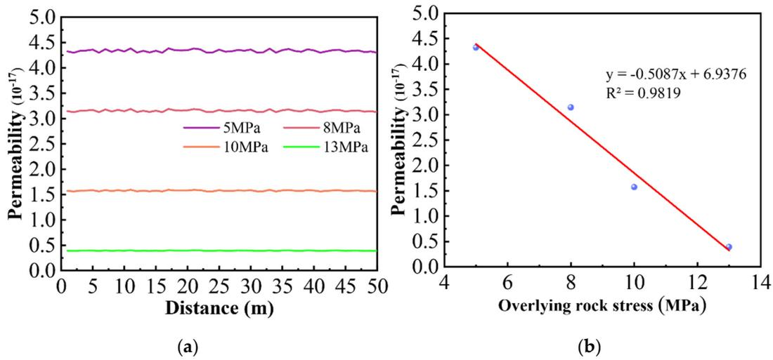
**Figure 7.** Variation in permeability of coal seams. (a) Stress permeability of different overburden rocks. (b) Stress and permeability fitting curves.
