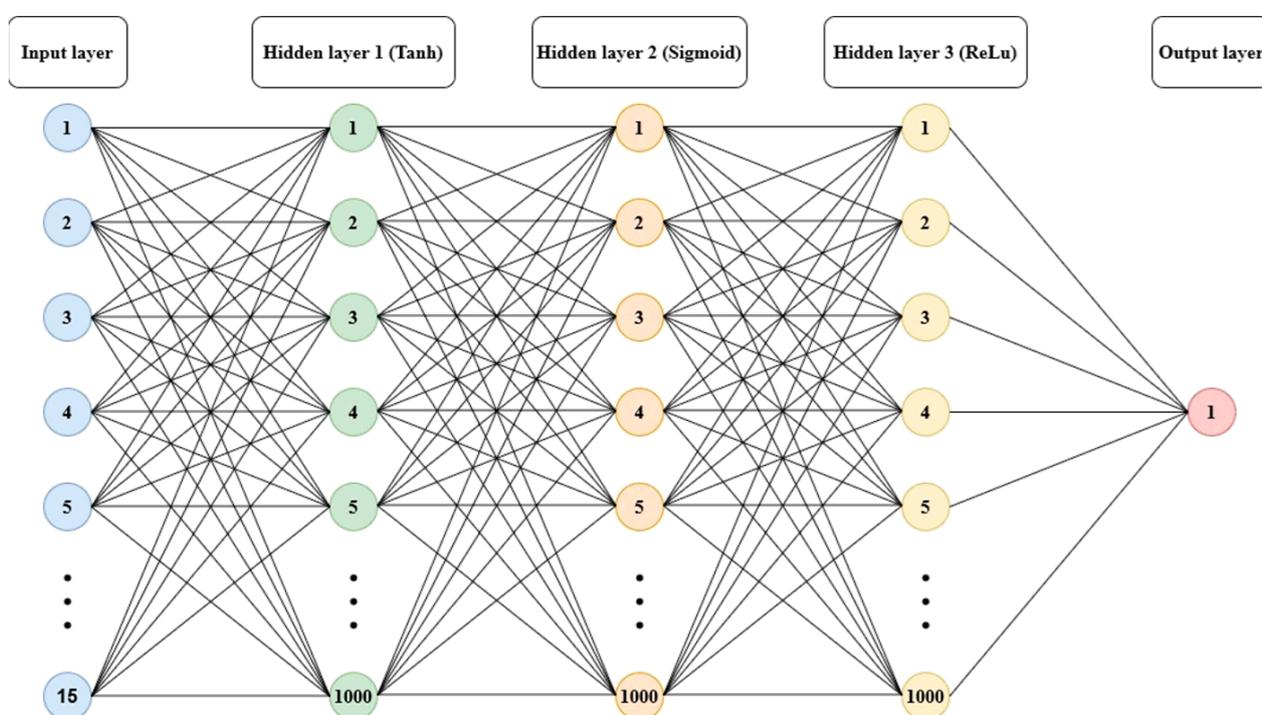
**Figure 1.** Model structure of the artificial neural network used. Input layer with 15 variables, representing the dependent variables, 3 hidden layers with 1000 neurons each, and the output layer with 1 variable ( $FV_{imb}$ ), representing the independent variable.
