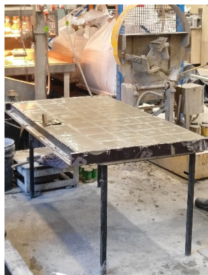
Figure 2. Timber mold used to cast samples.
