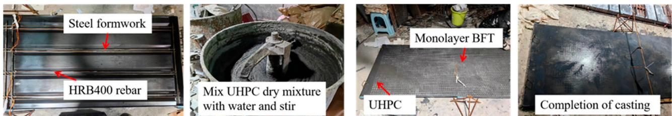
**Figure 8.** Specimen manufacturing process.
