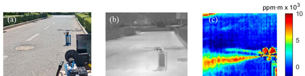
**Figure 14.** (a) Experimental scene; (b) gas release image; (c) gas column concentration inversion image.
