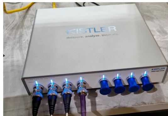
Figure 4. The used digital meter with the ability to record measurements, Kistler LabAmp type 5165A4KH00.
