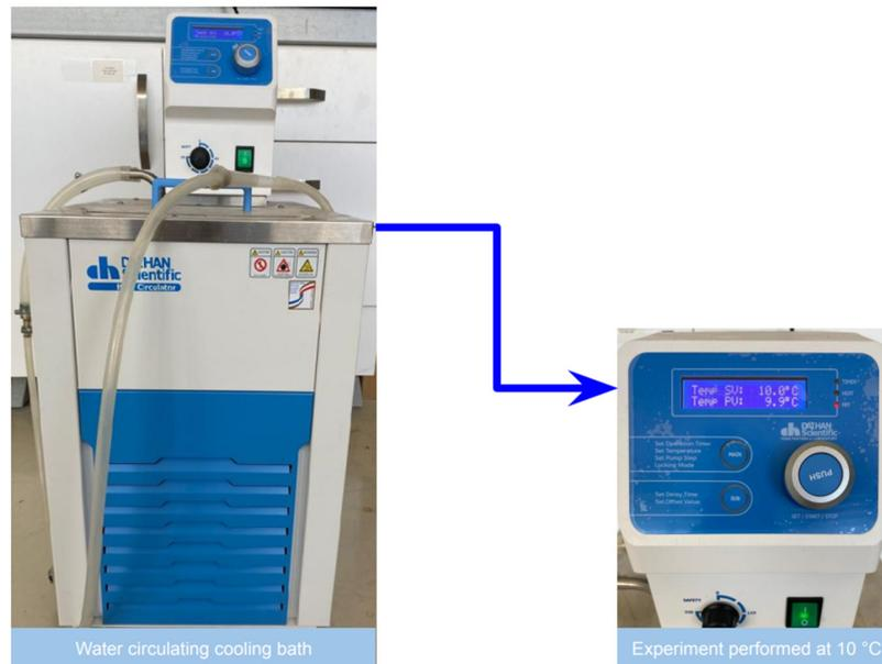
**Figure 2.** Water-circulating cooling bath with battery capacity experiment at 10 °C.
