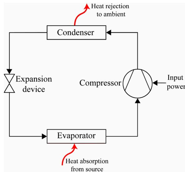
**Figure 10.** Schematic of a basic VCR cycle.
