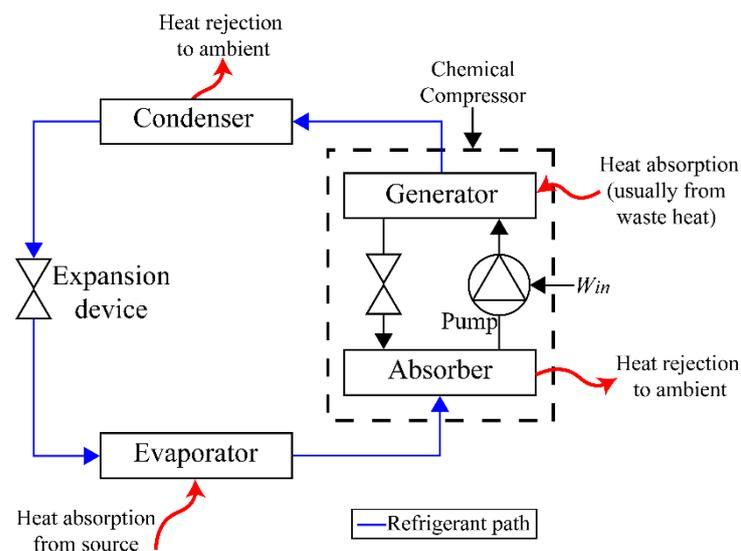
**Figure 7.** Schematic diagram of an absorption refrigeration system.
