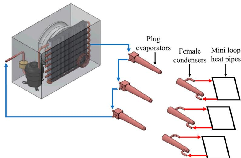
**Figure 14.** Illustrative representation of the hybrid cooling system.
