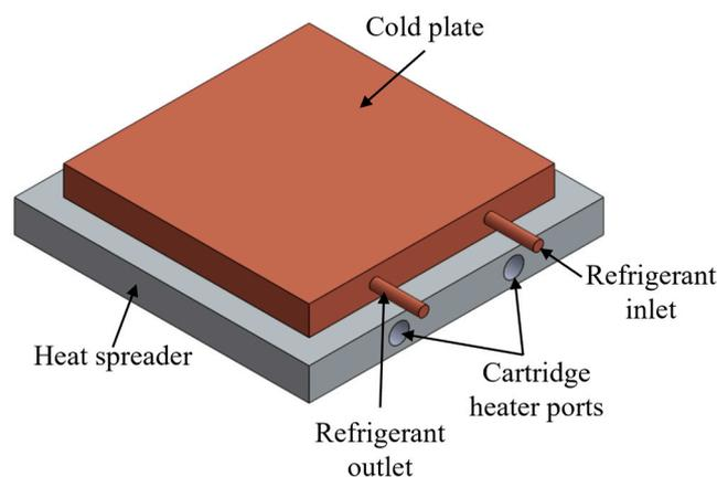
**Figure 26.** Illustrative representation of a small cold plate mounted on a heat spreader.
