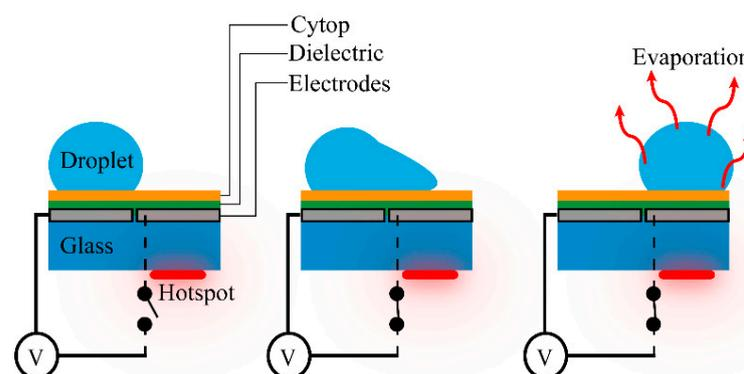
**Figure 4.** Schematic of electrowetting cooling.
