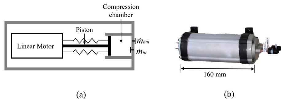
**Figure 20.** (a) Schematic of a linear compressor and (b) miniature linear compressor used by Ribeiro [54].
