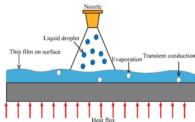
**Figure 2.** Schematic of spray cooling.
