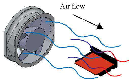
**Figure 1.** Schematic of forced convection heat transfer over a hot device.
