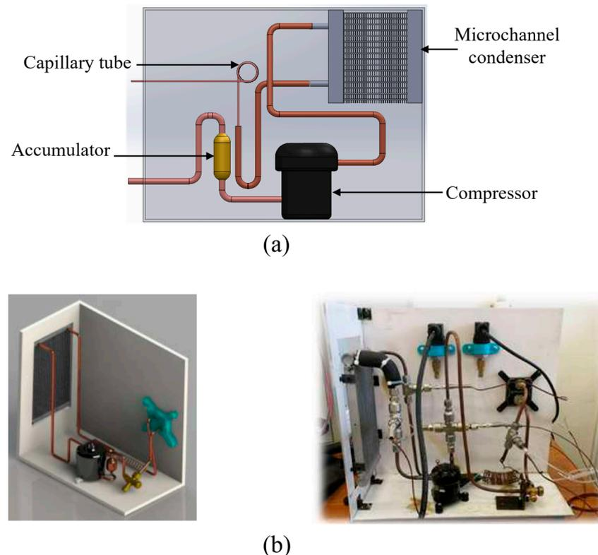
**Figure 11.** Experimental equipment of (a) Wu and Du and (b) Poachaiyapoom et al. [46].
