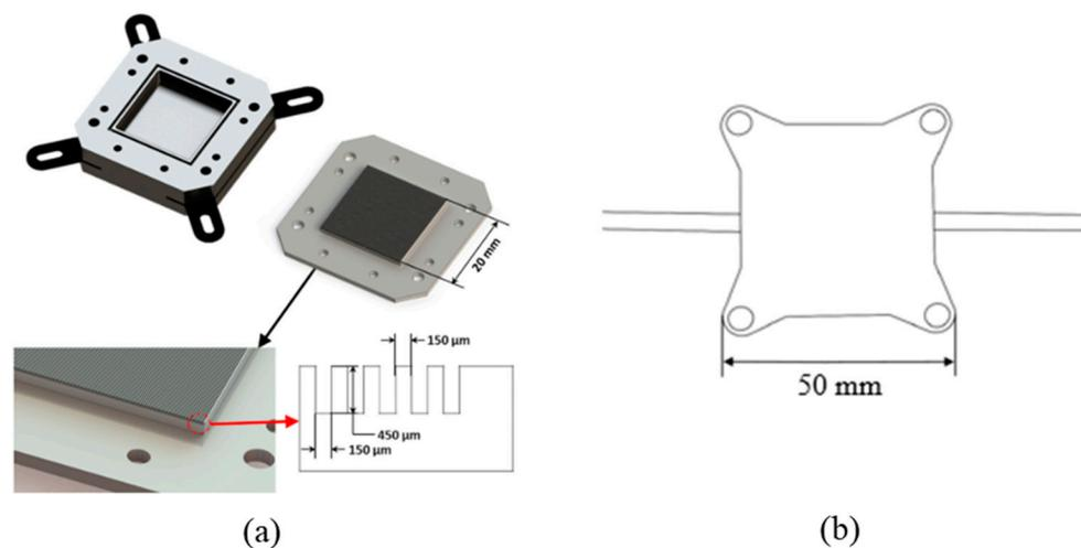
**Figure 24.** Miniature microchannel evaporators used by (a) Pochaiyapoom et al. [46] and (b) Mongia et al.
