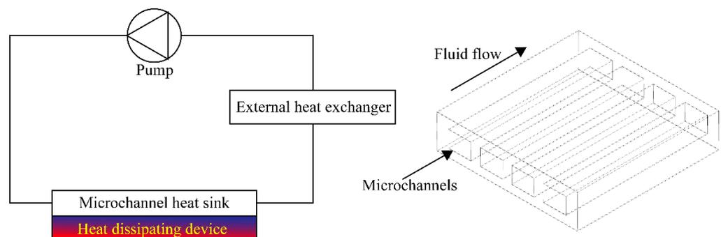
**Figure 6.** Schematic of a microchannel cooling system.
