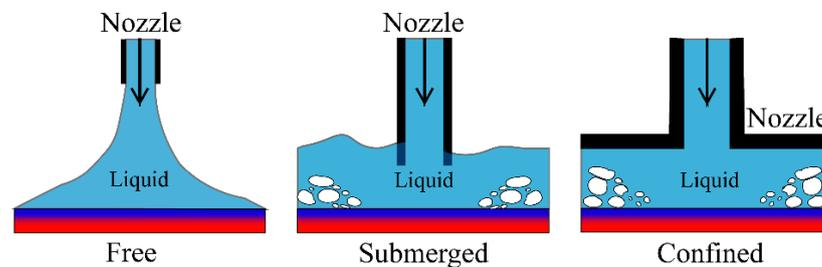
**Figure 3.** Schematic of jet impingement.
