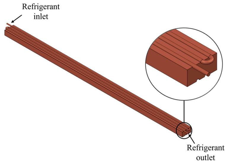
**Figure 27.** Illustrative representation of the cold plate.
