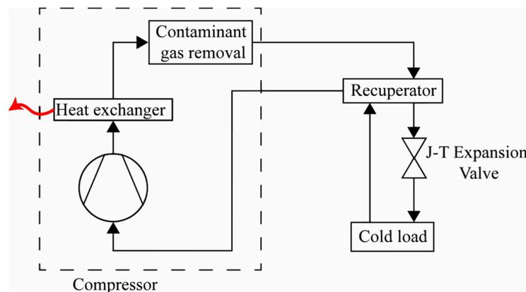
**Figure 9.** Schematic of a basic closed J-T cycle.
