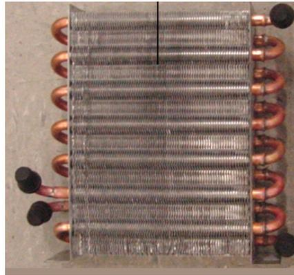
**Figure 22.** Finned-tube condenser used by Ribeiro [54].
