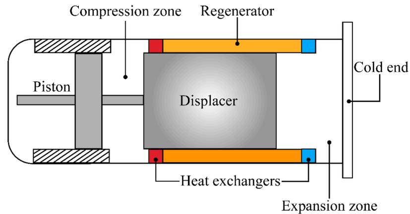
**Figure 8.** Schematic of Stirling cooling technology.
