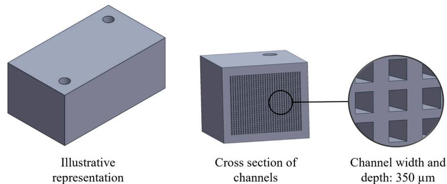
**Figure 25.** Illustrative representation of the microchannel plate-fin evaporator.
