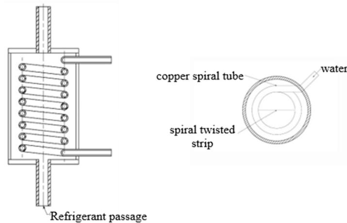
**Figure 23.** Illustrative representation of the miniature spiral-tube type evaporator.
