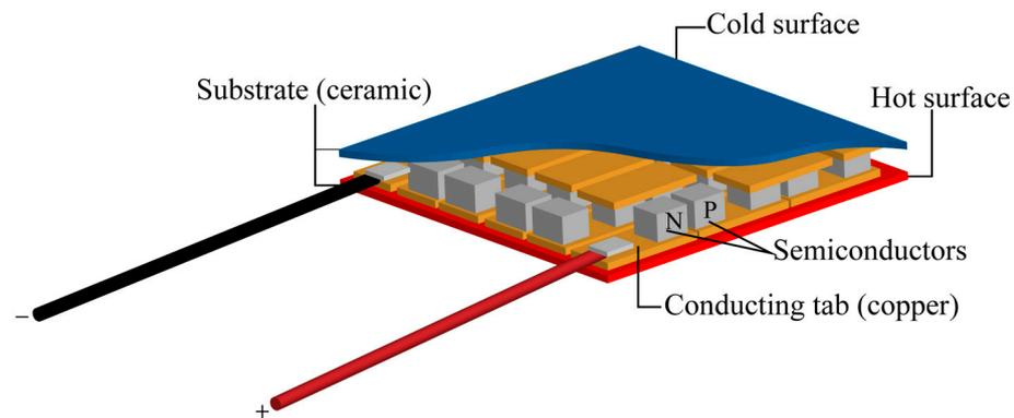
**Figure 5.** Schematic of thermoelectric cooler.
