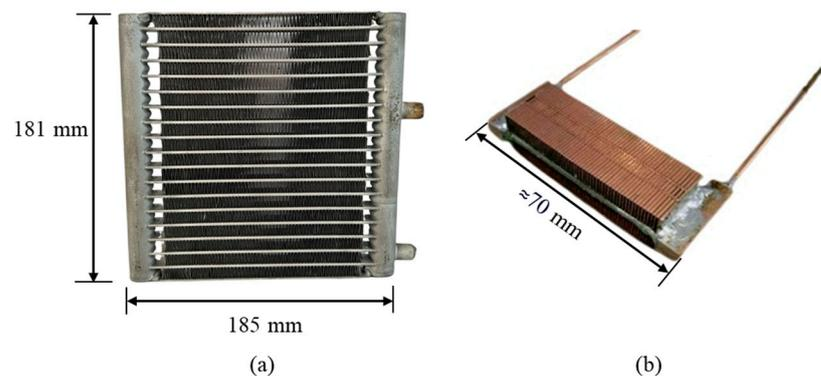
**Figure 21.** Microchannel condensers: (a) design 1 and (b) design 2.
