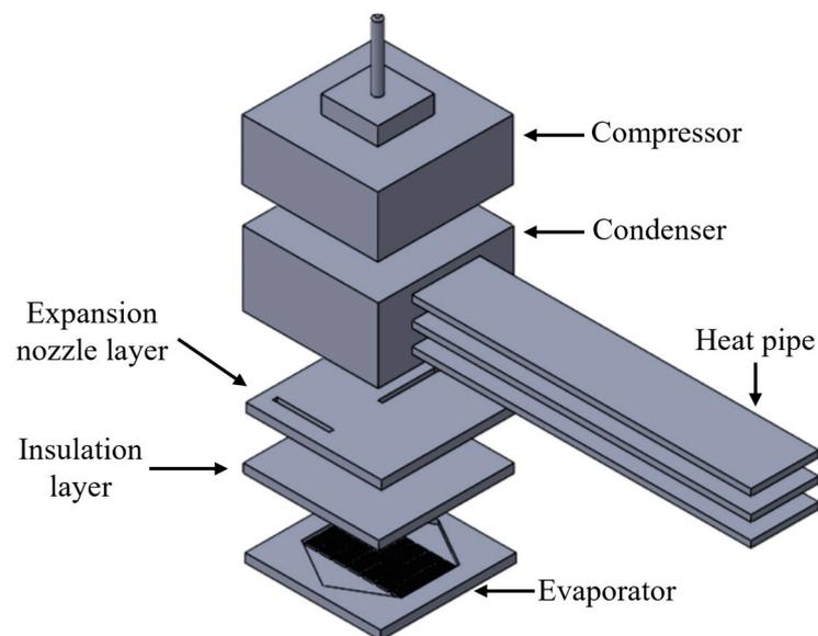
**Figure 15.** Illustrative representation of the meso-scale VCR system.
