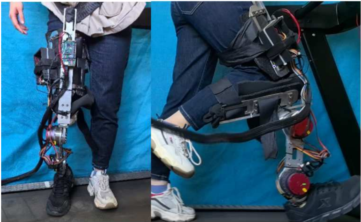
Figure 1. The intelligent prosthesis prototype being worn by a subject. The sensors include IMU and a foot-pressure sensor. Two motors are located on the knee and ankle joints.
