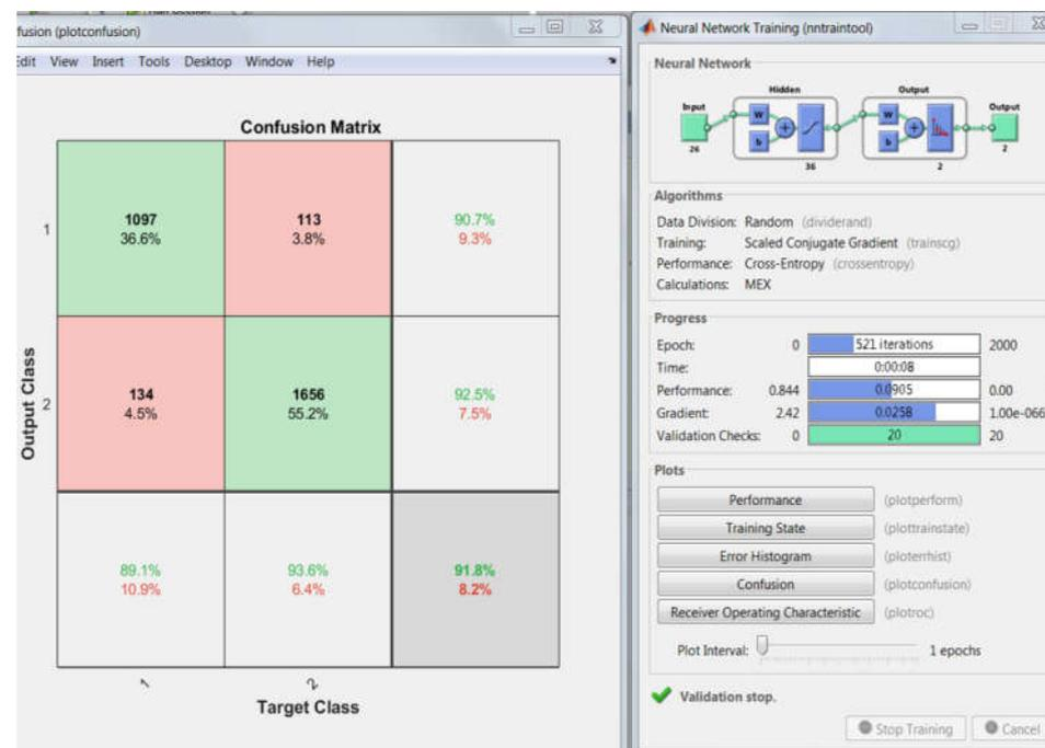
**Figure 2.** The confusion matrix for a 2-class classification (VF vs. another class) and the structure of the MLP neural network (Recall = 89.10%; Specificity = 93.68%; Error Rate = 8.23%; Precision = 90.74%; F1 score = 89.98%).
