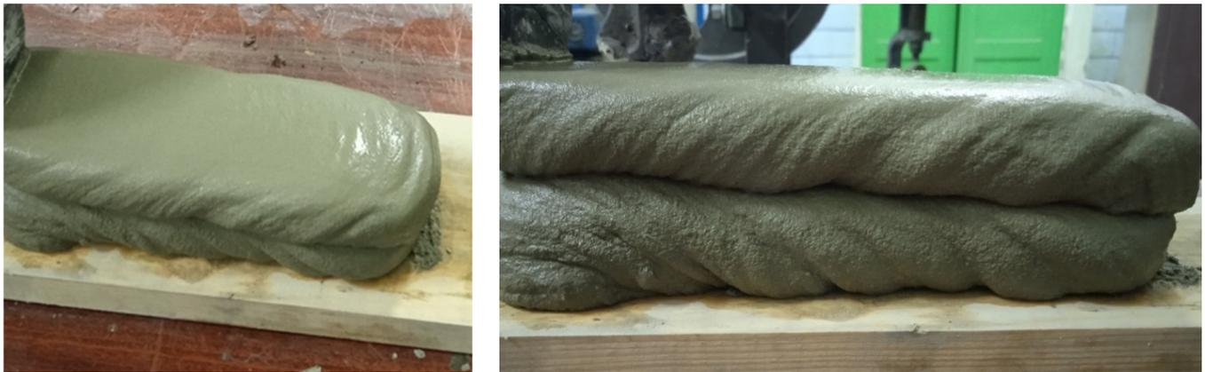
Figure 5. Photograph showing the test samples were made using a 3D printer.
