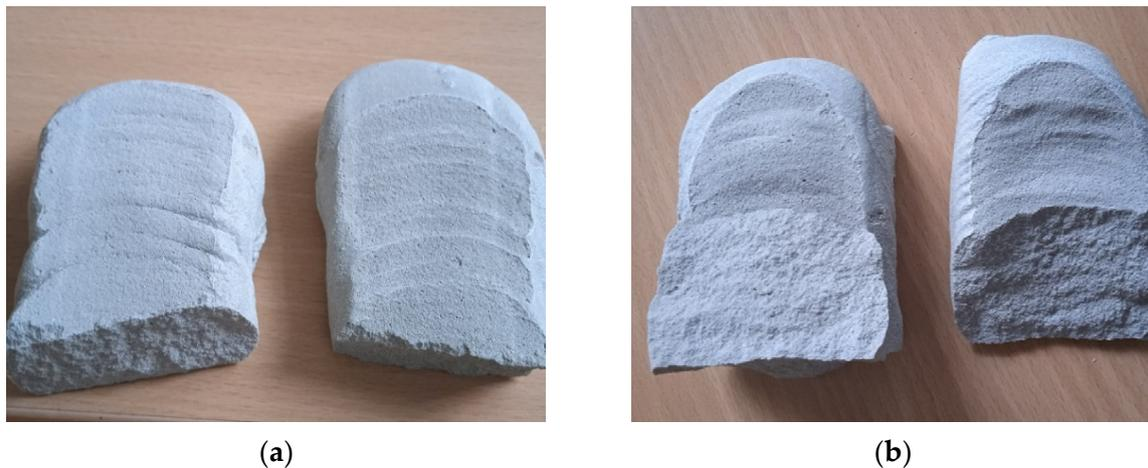
**Figure 15.** Destruction of samples during the determination of splitting strength: (a) destruction along the boundary of superimposed layers (slag–alkaline binder, composition No. 5, Table 6); (b) destruction beyond the boundaries of superimposed layers (cement–ash binder, composition No. 2, Table 6).
