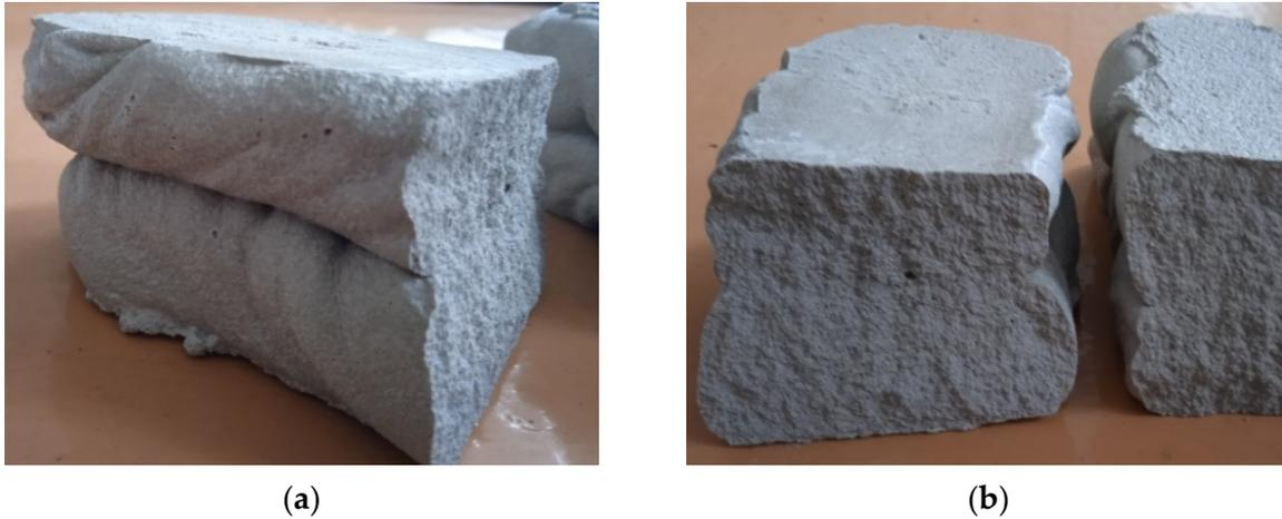
**Figure 14.** Destruction of samples during the determination of bending strength for slag–alkaline (a) and the cement–ash binders (b).
