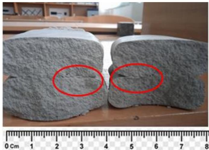
**Figure 1.** Photograph showing the defects when applying layers. Bonding zone—in red.
