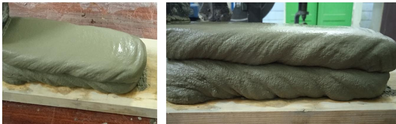
**Figure 5.** Photograph showing the test samples were made using a 3D printer.
