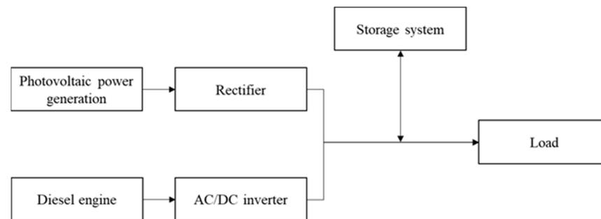
**Figure 1.** Mobile microgrid structure.
