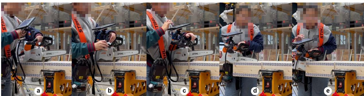
**Figure 16.** Evaluation of the TTool pipeline for chainsaw: (a) The user clips the display and sensor to the tool. (b) The camera is adjusted to include a chainsaw’s plate in the frame. (c) The tool is first detected by AI, and the pose is initialized by the user and refined automatically. (d) The user inserts the tool into the manufactured slot. (e) Finally, the pose is exported to a disk for later analysis.
