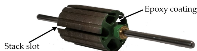
Figure 2. Epoxy coating addition sub-process.
