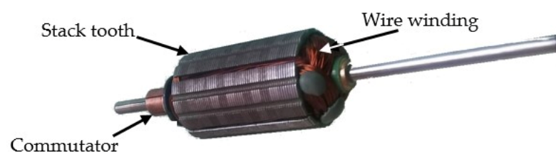
Figure 3. Sub-process of magnetic wire winding.
