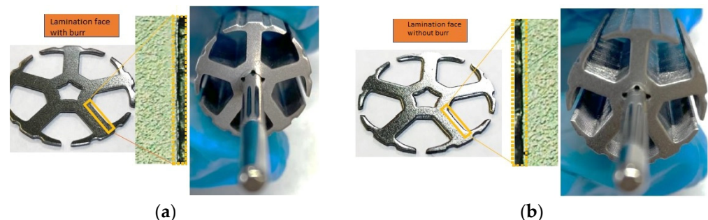
Figure 21. Lamination face (a) with burr and (b) without burr.
