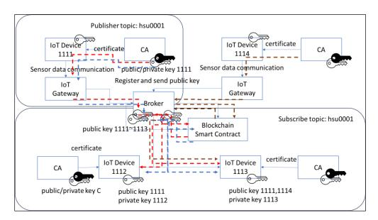
Figure 9. Added 1111 key broadcast to provide node 1113 with three keys.
