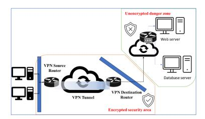
Figure 2. Vulnerabilities in using VPN to encrypt communications.
