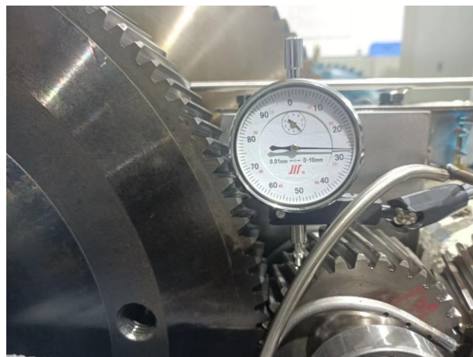
Figure 11. Dual-input counter-rotating gearbox backlash measurement physical diagram.
