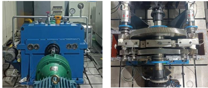
Figure 10. Dual-input counter-rotating gearbox test stand.
