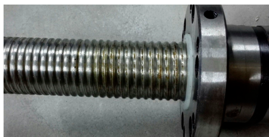
Figure 1. Agglomeration phenomenon of lubricating grease after long-term storage.
