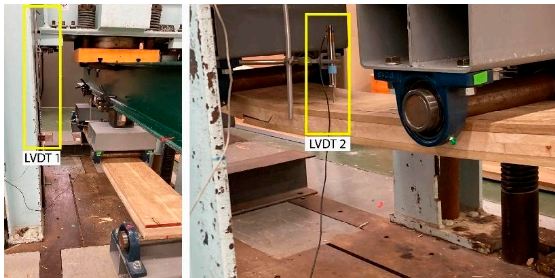
Figure 7. Actual testing arrangement for DCLT bending specimens.
